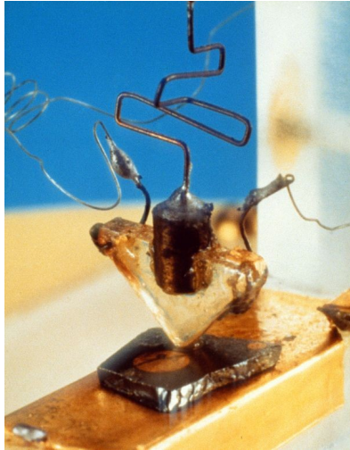
Figure 2.5: Bardeen and Brattain's first point-contact transistor (1947). Image from the Computer History Museum's website , Copyright Alcatel-Lucent USA Inc.
