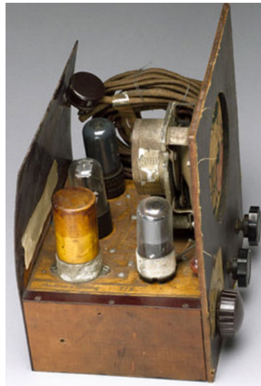
Figure 2.7: Radio with the first Printed Circuit Board (PCB) by Paul Eisler (1942). Image from the Science & Society Picture Library website . Copyright Science Museum / Science & Society Picture Library.
