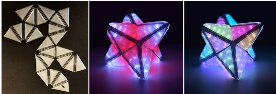
Figure 3.26: 3D printed light diffuser for the star model (left). Light effects on the design: inside-out pulse (middle) and per triangle colors (right).
