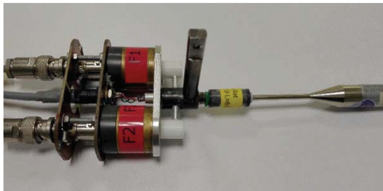
Fig. 3 [Probe/cavity/reference microphone] assembly for calibration
