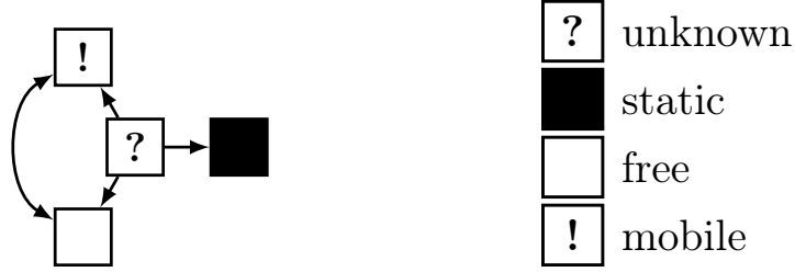
Figure 5.2: Cell occupancy status transition diagram.
