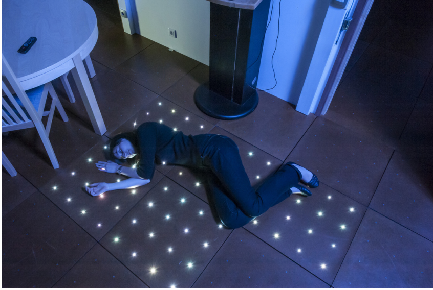
Figure 3.17 – The floor detects and localises hard falls using its accelerometers
