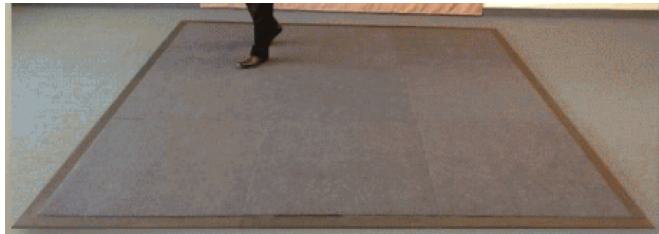
Figure 2.23 – The GAITRite Surface pressure-sensing floor [50]
