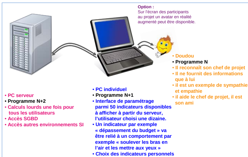
Figure 91 : Architecture hardware (notre recherche)
