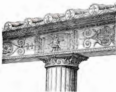
Fig. 89.—Colonnade of the Stabian Baths: capital with section of entablature, restored.
