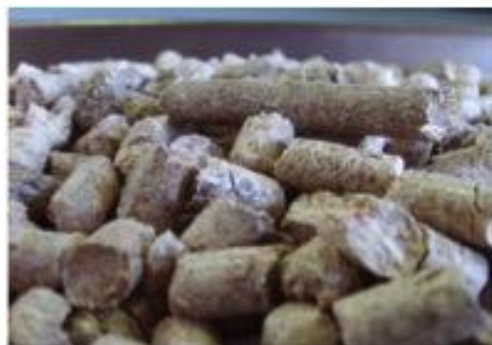
Figure 9: MXG pellet (6 mm of diameter)
