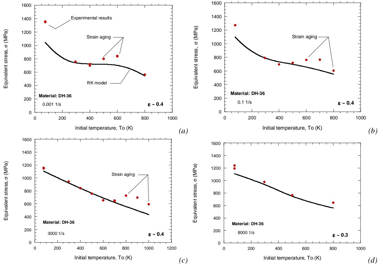
Fig. 2.6. Temperature sensitivity description of the steel **DH-36** by the **RK** model, comparison with experimental results for  $\epsilon_p=0.4$  [Nemat-Nasser and Guo, 2003]. (a)  $0.001 \text{ s}^{-1}$ , (b)  $0.1 \text{ s}^{-1}$ , (c)  $3000 \text{ s}^{-1}$ , (d)  $8000 \text{ s}^{-1}$ .
