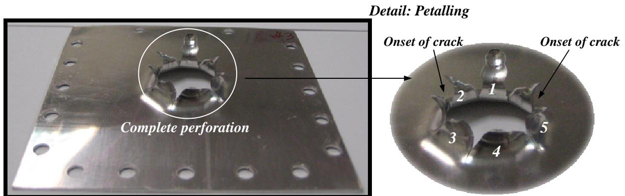
Fig. 4.56. Petalling failure mode for  $V_0 = 2.0 \text{ m/s}$  and  $T_0 = 213\text{K}$ .
