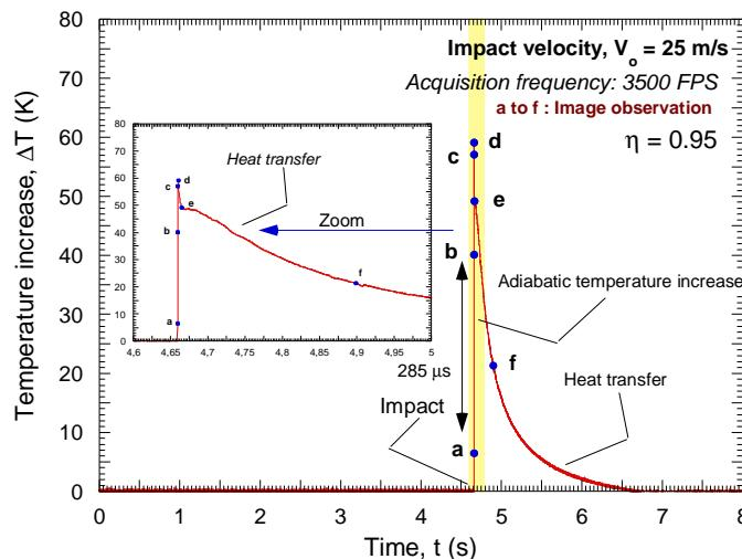
Fig. 4.21. Evolution of the maximum increase of temperature in the target as a function of time,  $V_0 = 25 \text{ m/s}$ .
