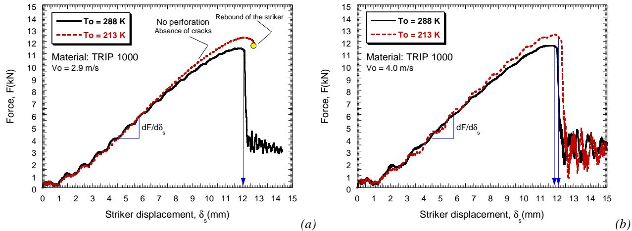
Fig. 5.58. Evolution of the force versus the striker-displacement for both initial temperatures.
