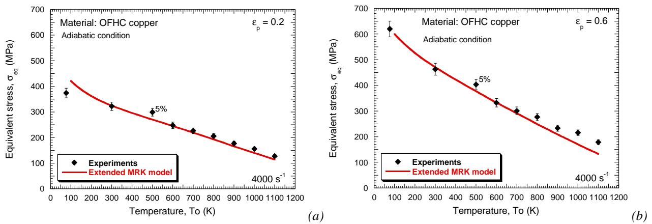
Fig. 2.33. Temperature sensitivity description using the extended MRK model and comparison with experiments at  $4000\text{ s}^{-1}$ . (a)  $\varepsilon_p=0.2$ , (b)  $\varepsilon_p=0.6$  [Nemat-Nasser and Li 1998].
