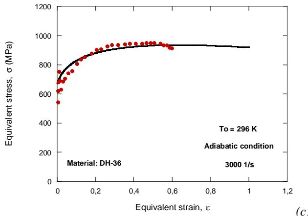
Fig. 2.4. Comparison between analytical predictions (this Thesis) and experimental results for the steel DH-36 [Nemat-Nasser and Guo, 2003] for different strain rate levels at room temperature. (a)  $0.001 \text{ s}^{-1}$ , (b)  $0.1 \text{ s}^{-1}$  (c)  $3000 \text{ s}^{-1}$ .
