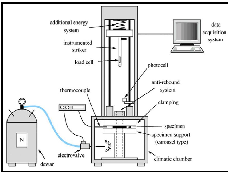
Fig. 4.45. Schematic representation of the drop weight tower (UC3M) [Gómez-del Río et al. 2005].
