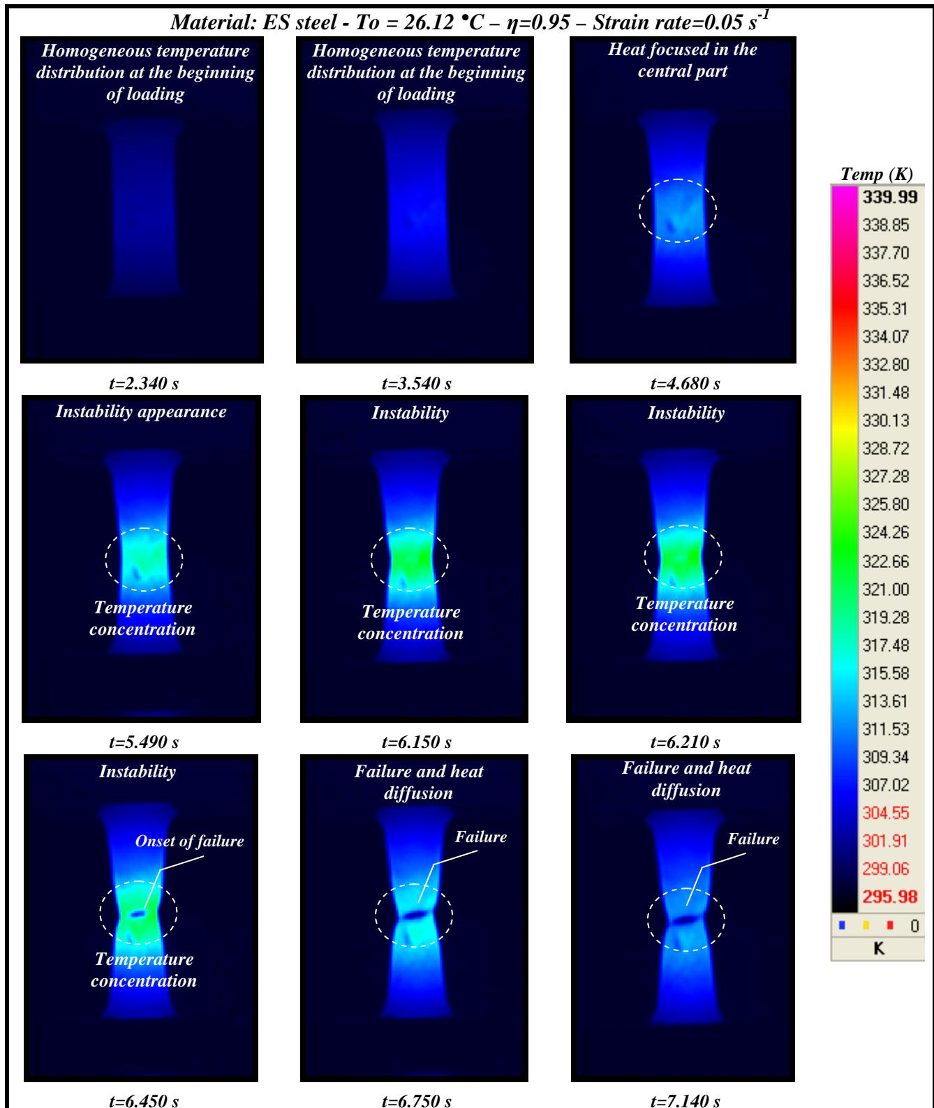
Fig. 4.9. Temperature contours during loading. Picture resolution 320×256 pixels.
