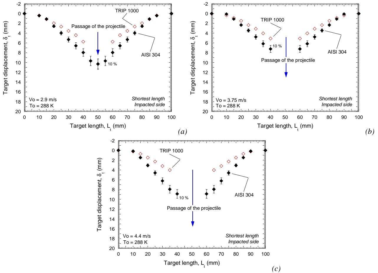
Fig. 5.54. Permanent bending of the target. Comparison between AISI 304 and TRIP 1000 for different impact velocities.
