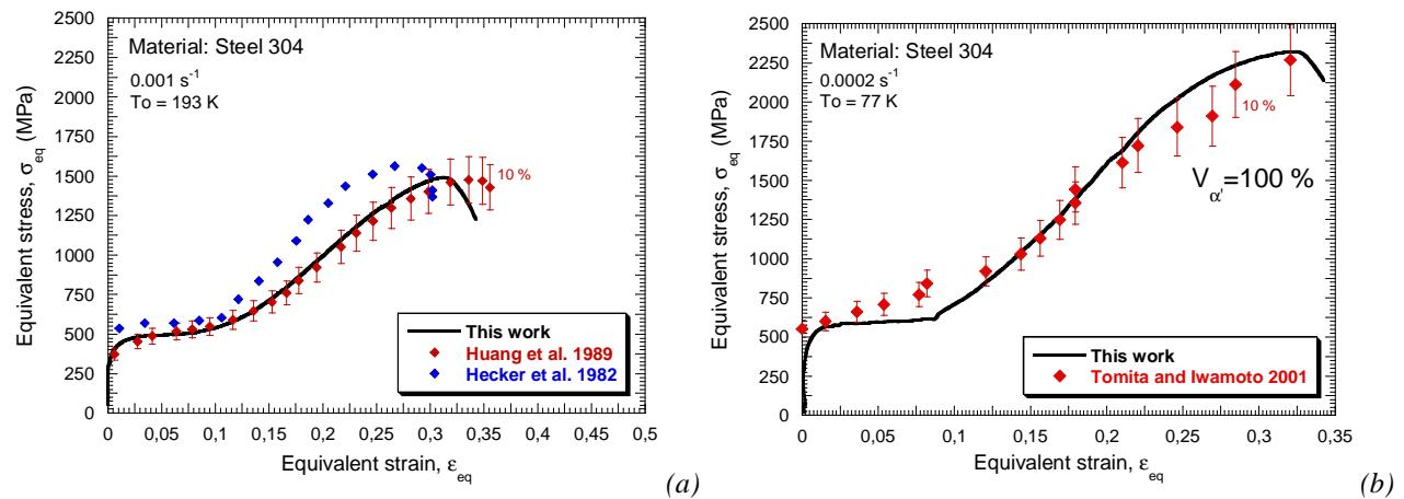
Fig. 5.20. Flow stress evolution versus plastic strain at low strain rates. (a)  $T_0 = 193$  K, (b)  $T_0 = 77$  K. Comparison with experimental results [Huang et al. 1989, Hecker et al. 1992, Tomita and Iwamoto 2001]
