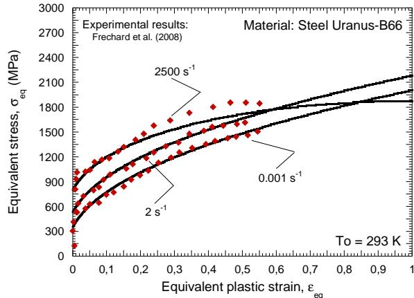
Fig. 2.15. Flow stress evolution as a function of plastic strain for different strain rates. Comparison between modelling and experiments [Frechard et al. 2008].
