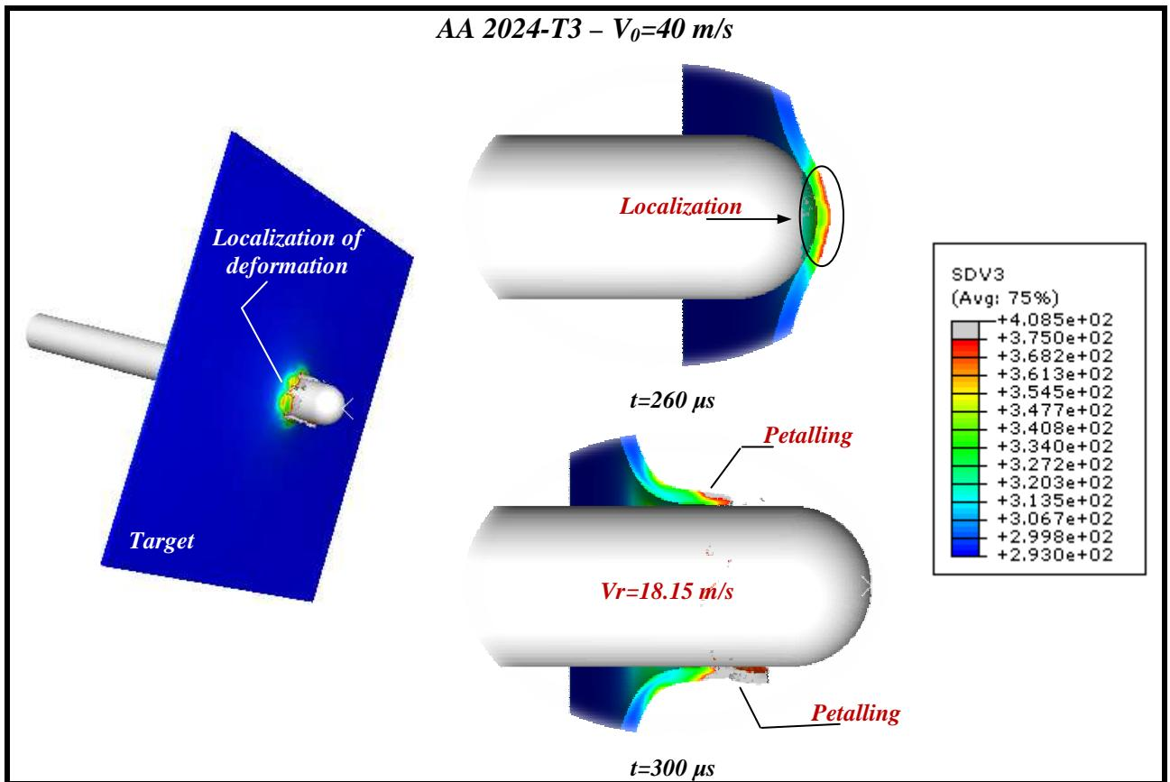
Fig. 4.65. Numerical estimations of temperature contours during impact,  $V_0 = 40 \text{ m/s}$ .
