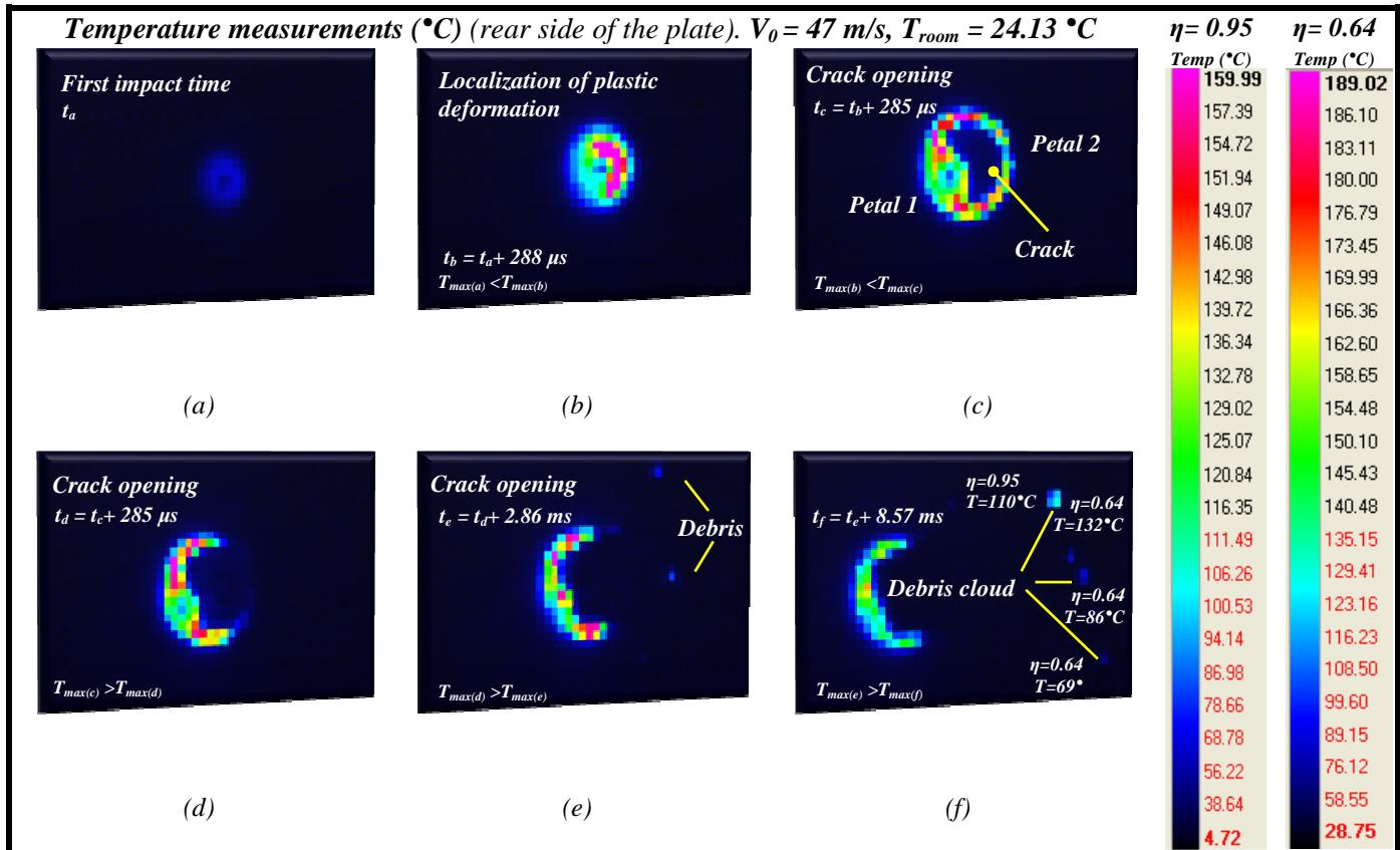
Fig. 4.24. Temperature level ( $^{\circ}\text{C}$ ) along the impact process for an impact velocity leading to target-perforation, observation of debris cloud,  $V_0 = 47 \text{ m/s}$  and  $T_{\text{room}} = 24.13 \text{ }^{\circ}\text{C}$ . Picture resolution  $80 \times 64$  pixels.
