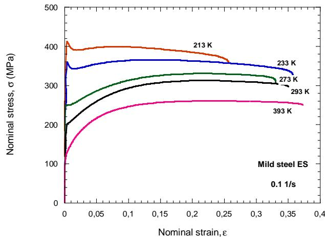
Fig. 4.4. Temperature effect on flow stress for mild steel ES at  $0.1 \text{ s}^{-1}$  [Rusinek et al. 2005].
