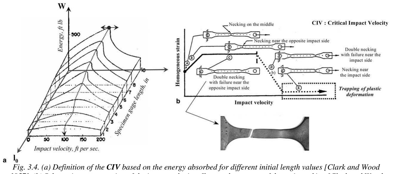
Fig. 3.4. (a) Definition of the **CIV** based on the energy absorbed for different initial length values [Clark and Wood 1957]. (b) Schematic representation of the impact velocity effect on the process of dynamic necking [Clark and Wood 1957, Rusinek et al. 2005].
