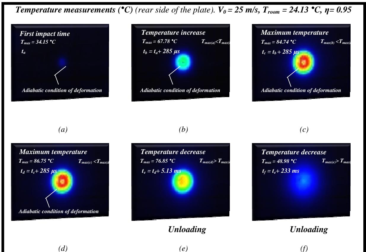
Fig. 4.20. Temperature in the rear side of the target for different stages of the impact process.
