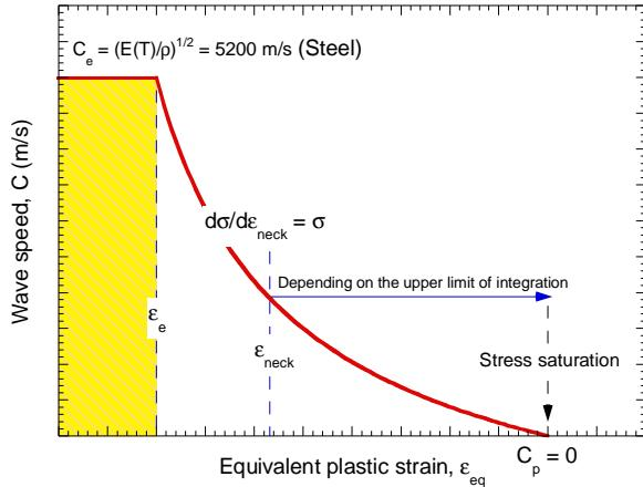
Fig. 3.5. Schematic representation of the wave speed as a function of plastic strain for determined strain rate and temperature levels. Influence of the upper limit of integration  $\epsilon_{pm}$  on the CIV value.
