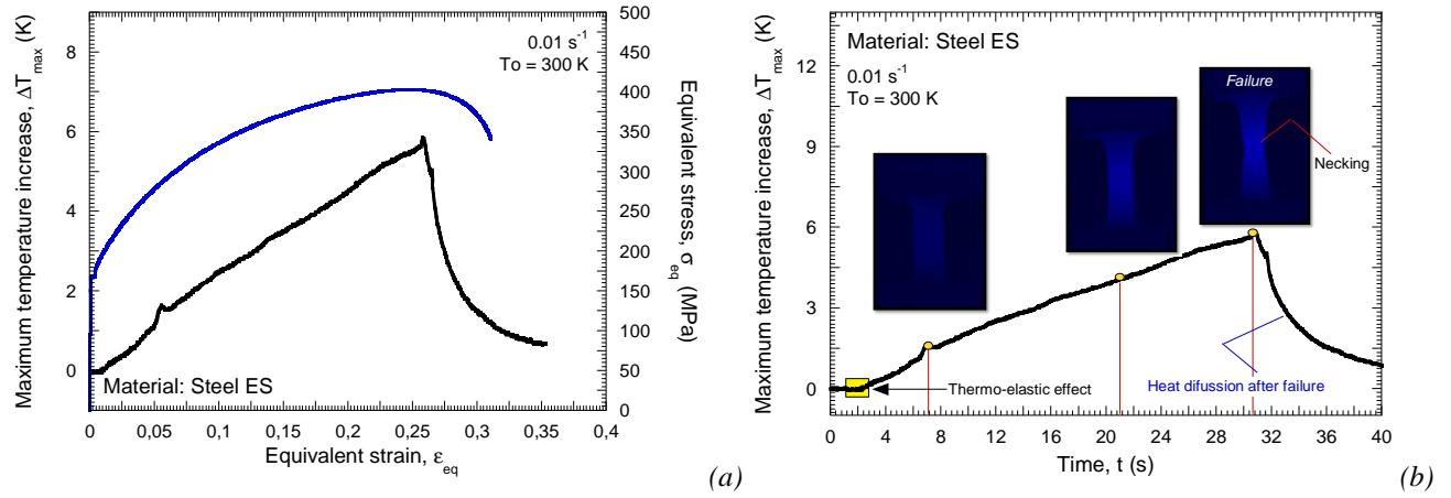
Fig. 4.6. (a) Maximum temperature increase versus plastic strain and flow stress evolution versus plastic strain.
