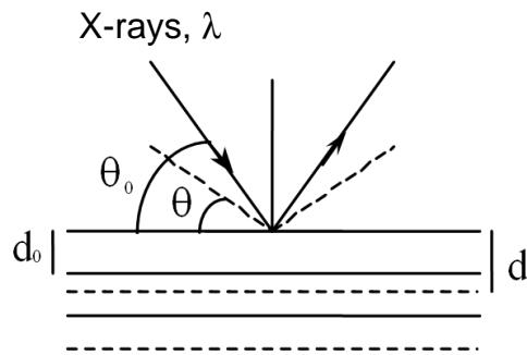
Fig. 5.1. Principle of X-ray diffraction ( $d_0$  and  $\theta_0$  are respectively the lattice spacing and the Bragg angle corresponding to a stress free state).
