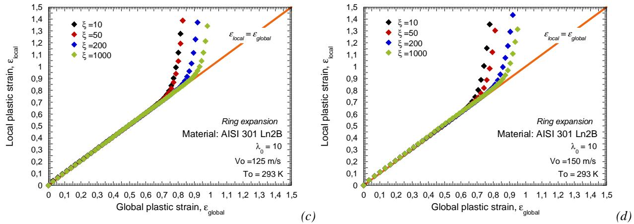
Fig. 3.80. Evolution of the local plastic strain with the global plastic strain for the configurations analyzed
