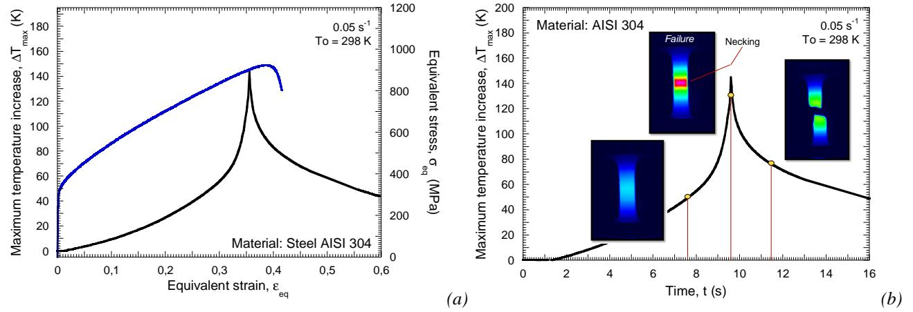
Fig. 5.14. (a) Maximum temperature increase versus plastic strain and flow stress evolution versus plastic strain.
