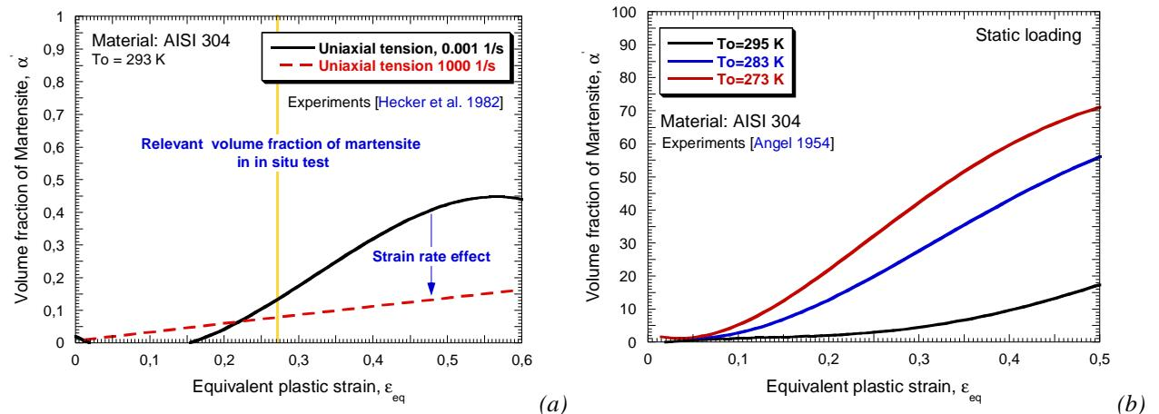
Fig. 5.10. (a) Actual volume fraction of martensite formed during straining at room temperature in tension at low and high strain rate at room temperature [Hecker et al. 1982]. (b) Formation of martensite by tensile plastic strain at various deformation temperatures [Angel 1954].
