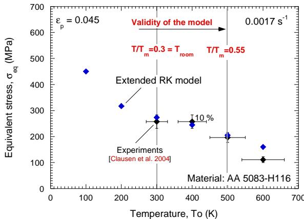
Fig. 2.41. Description of the temperature sensitivity by the extended **RK** model and comparison with experiments for  $\varepsilon_p=0.045$  and  $0.00017 \text{ s}^{-1}$  [Clausen et al. 2004].
