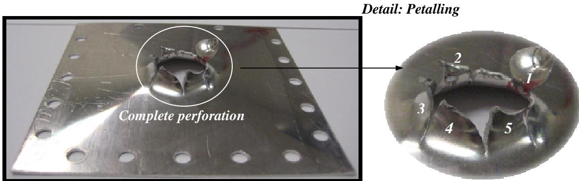
Fig. 4.55. Petalling failure mode for  $V_0 = 4.0 \text{ m/s}$  and  $T_0 = 213\text{K}$ .
