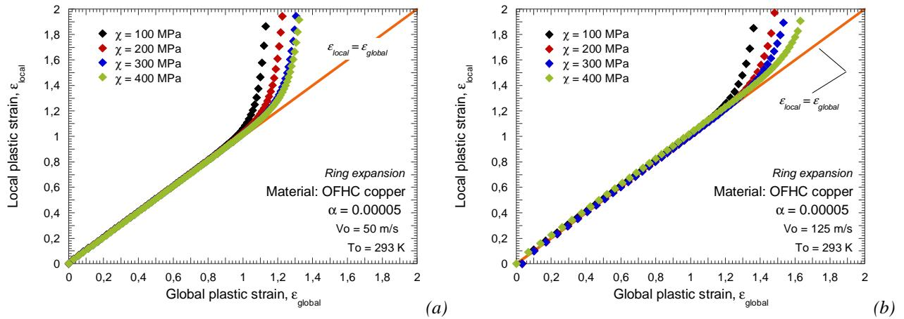
Fig. 3.32. Evolution of the local plastic strain versus the global plastic strain for different values of  $\chi$ .
