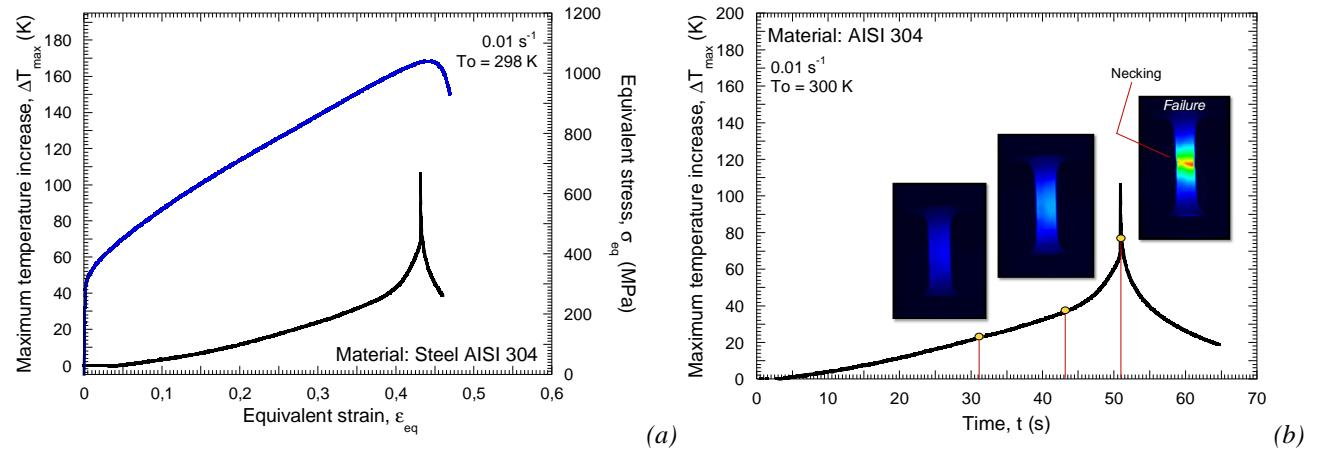
Fig. 5.12. (a) Maximum temperature increase versus plastic strain and flow stress evolution versus plastic strain.
