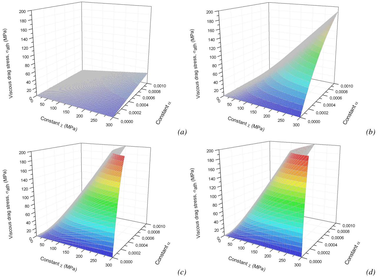
Fig. 2.28. Evolution of the viscous drag component as a function of  $\chi$  and  $\alpha$  for different strain rate levels.
