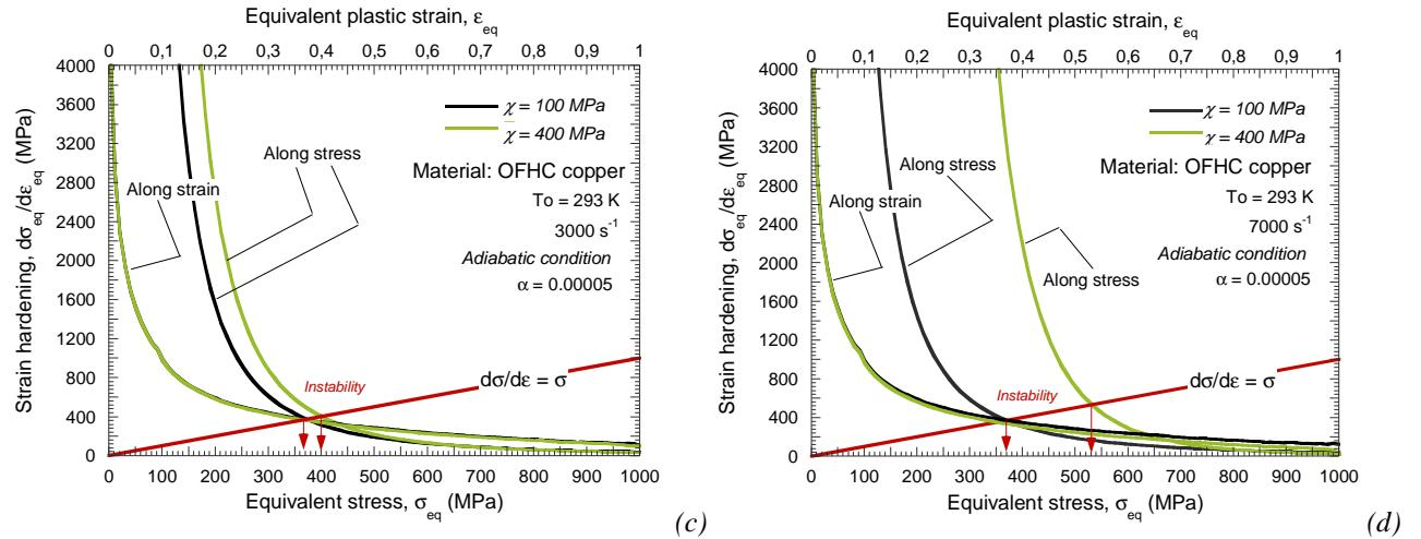
Fig. 3.31. (a)-(b) Flow stress evolution as a function of the plastic strain for different values of  $\chi$ . (c)-(d) Strain hardening evolution versus plastic strain and stress for different values of  $\chi$ .
