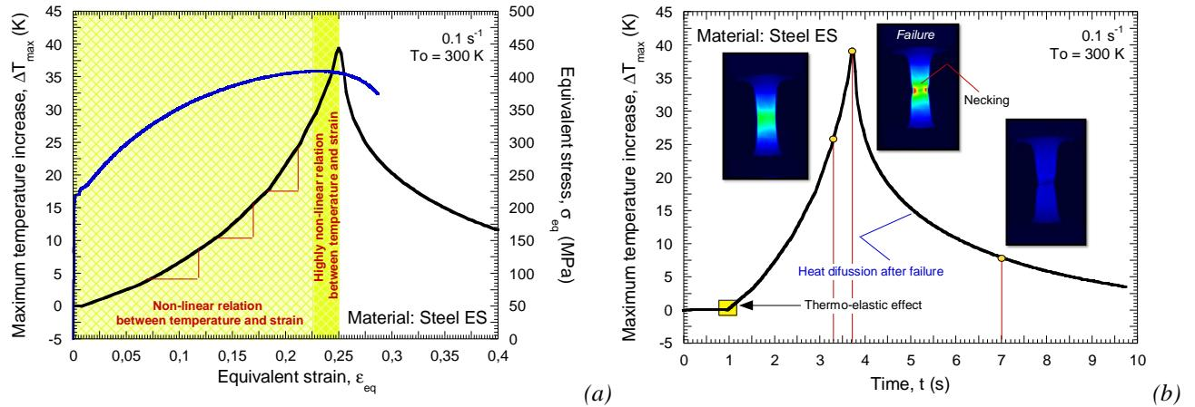
Fig. 4.10. (a) Maximum temperature increase versus plastic strain and flow stress evolution versus plastic strain.
