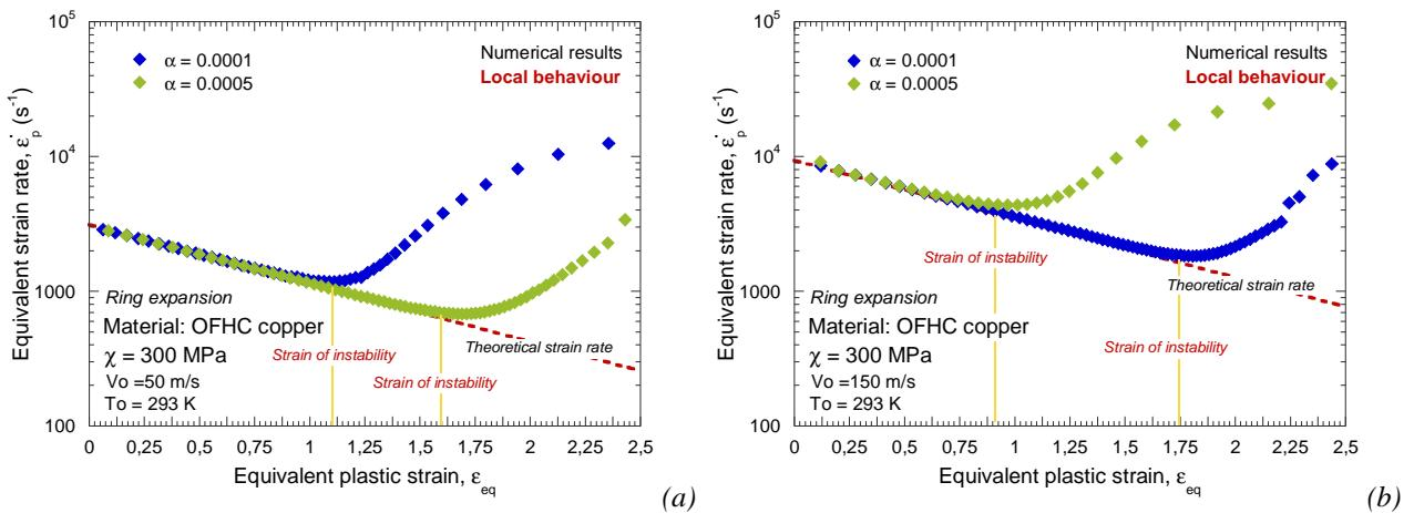
Fig. 3.49. Strain rate in the necking versus plastic strain in the necking in the case of  $\alpha=0.0001$  and  $\alpha=0.0005$ .
