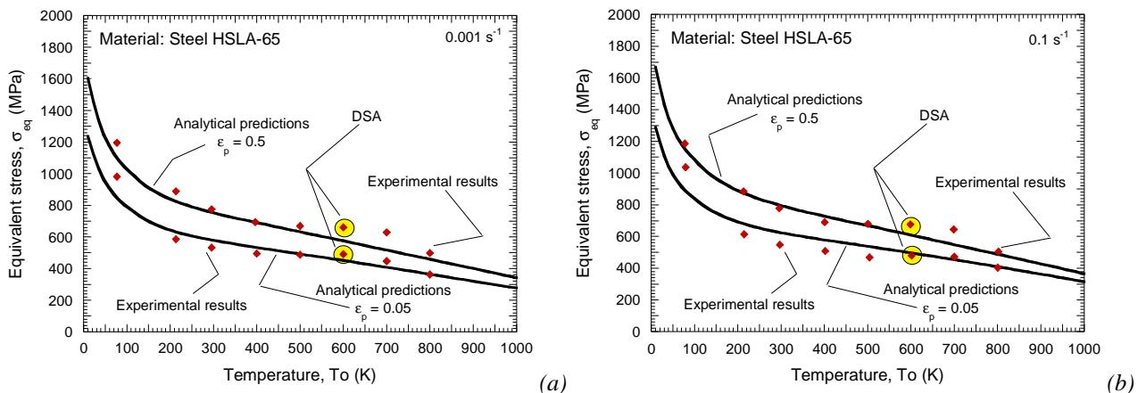
Fig. 2.9. Temperature sensitivity description of the steel HSLA-65 by the RK model, comparison with experimental results for  $\varepsilon_p=0.05$  and  $\varepsilon_p=0.5$  [Nemat-Nasser and Guo 2005]. (a)  $0.001 \text{ s}^{-1}$ , (b)  $0.1 \text{ s}^{-1}$ .
