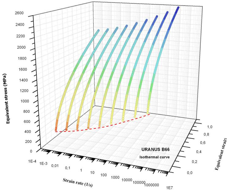
Fig. 2.19. Description of the flow stress of the steel alloy **Uranius-B66** predicted by the **RK** model within wide ranges of strain and strain rate.
