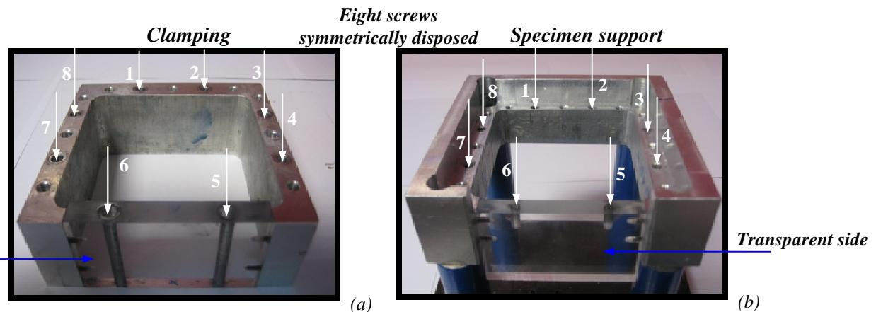
Fig. 4.46. Experimental device used to clamp the specimen during perforation tests (Design: S. Puerta and J. Puerta). (a) Clamping, (b) Specimen support.
