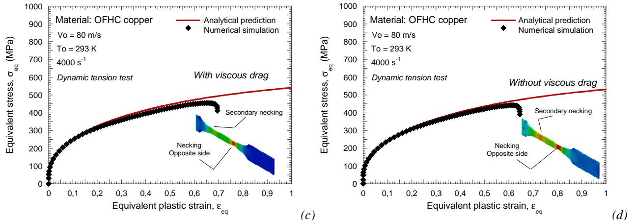
Fig. 3.17. Comparison between numerical results and analytical predictions for **MRK** and extended **MRK** models at different impact velocities,  $V_0 = 40 \text{ m/s}$  and  $V_0 = 80 \text{ m/s}$ .
