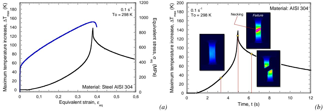
Fig. 5.16. (a) Maximum temperature increase versus plastic strain and flow stress evolution versus plastic strain.
