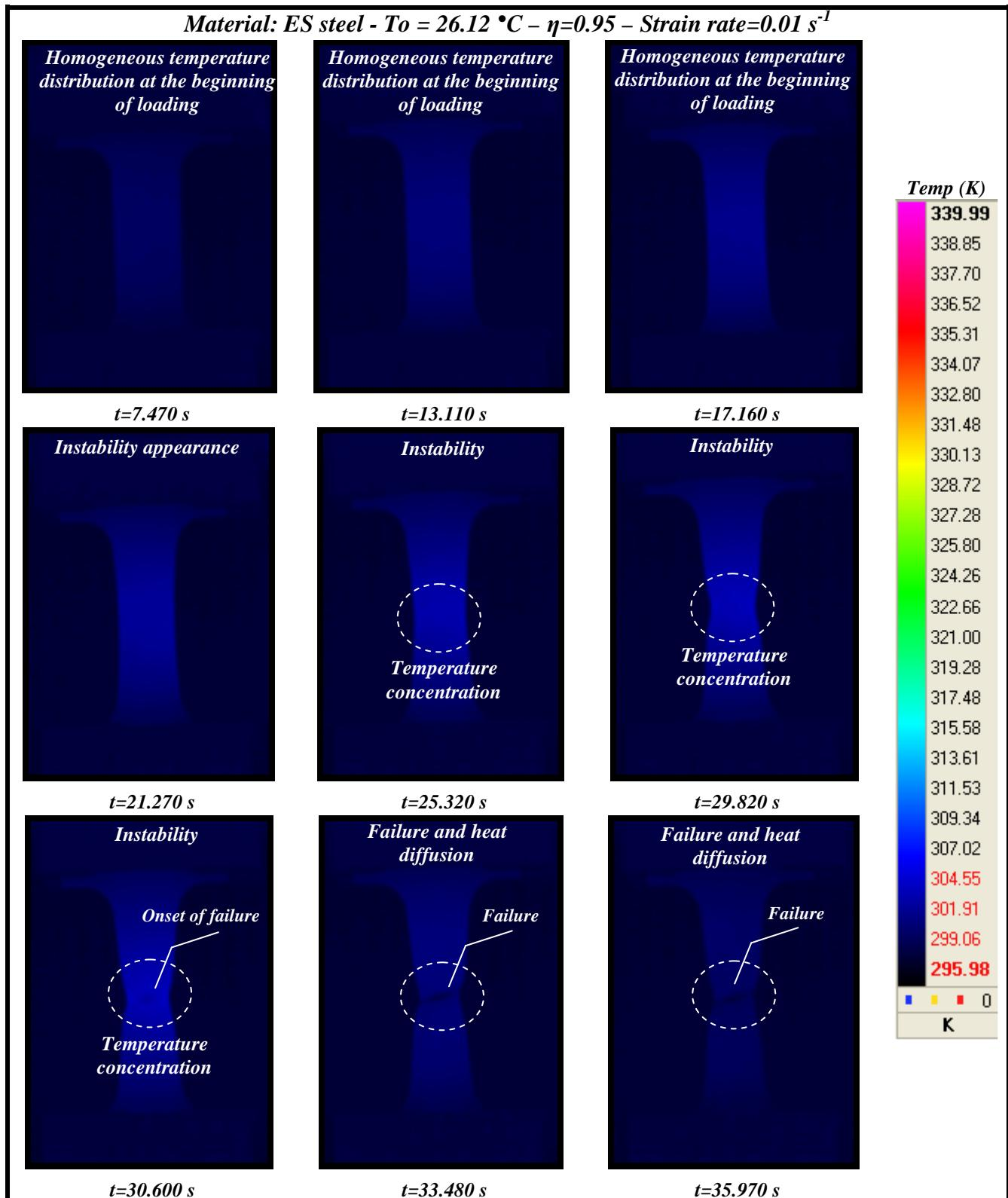
Fig. 4.7. Temperature contours during loading. Picture resolution 320×256 pixels.
