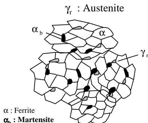
Fig. 5.42. Scheme of the microstructure of **L-TRIP** steel
