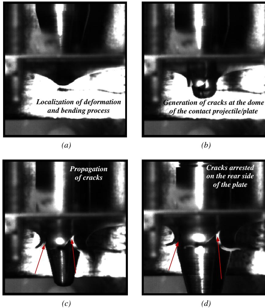
Fig. 5.50. Different stages of the perforation process for  $V_0=4.4 \text{ m/s}$  at room temperature. (a) Localization of deformation and bending process. (b) Generation of cracks at the dome of the contact projectile/plate. (c) Propagation of cracks. (d) Cracks arrested on the rear side of the plate.
