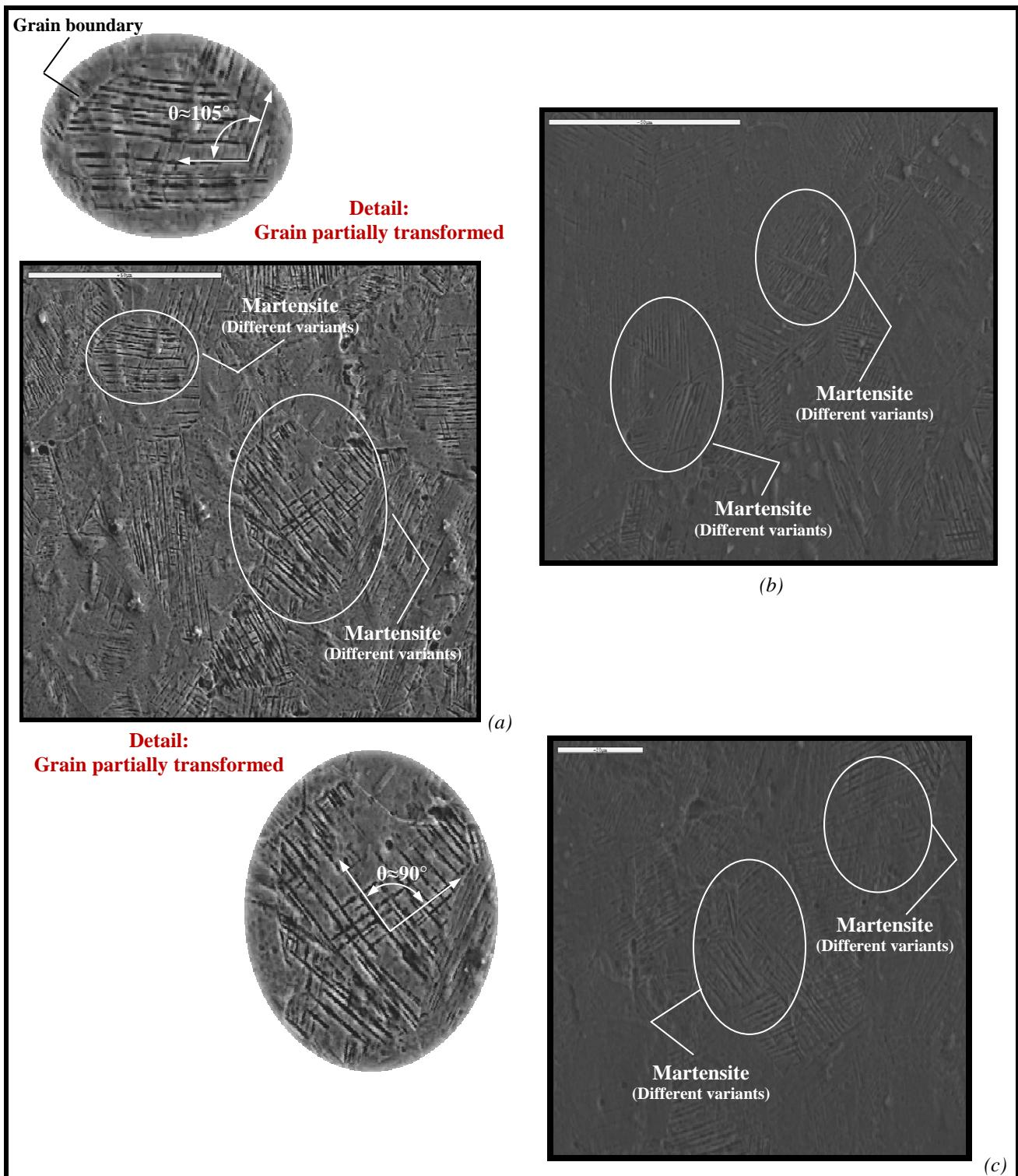
Fig. 5.28. SEM microographies of petals in AISI 304 impacted plates.(a)  $V_0=4.4 \text{ m/s}$ , (b)-(c)  $V_0=3.5 \text{ m/s}$ .
