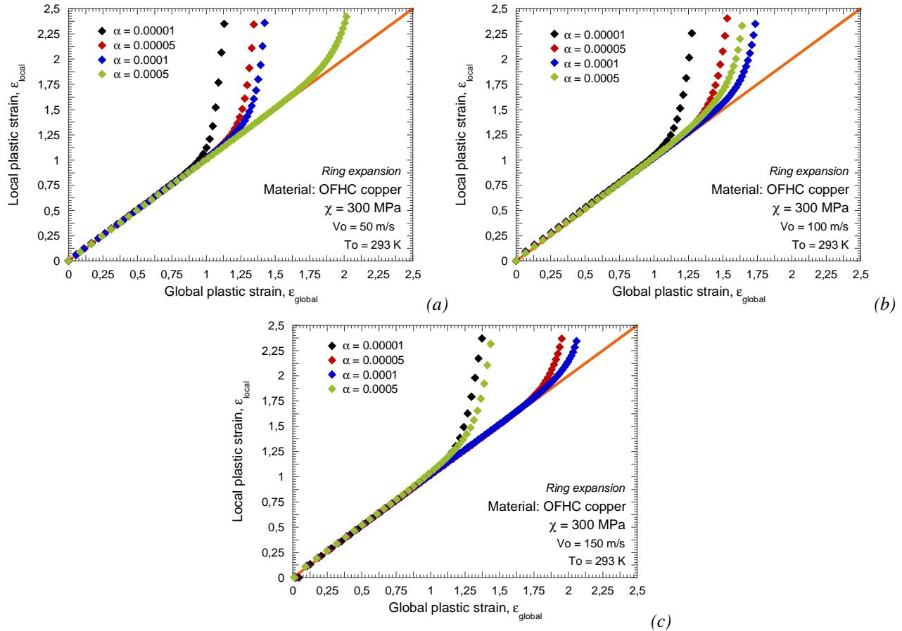
Fig. 3.47. Evolution of the local plastic strain as a function of the global plastic strain for different values of  $\alpha$ .
