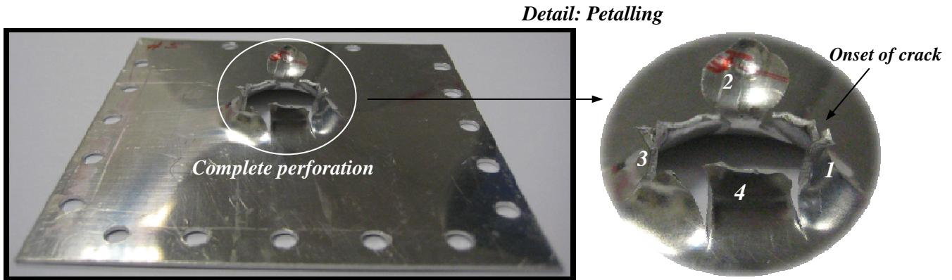
Fig. 4.51. Petalling failure mode for  $V_0 = 2.0\text{ m/s}$  and  $T_0 = 288\text{ K}$ .
