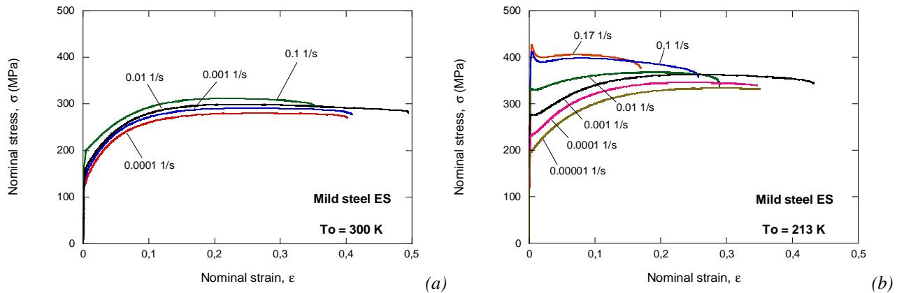
Fig. 4.3. Strain rate effects on the material flow stress. (a)  $T_0 = 300 \text{ K}$ , (b)  $T_0 = 213 \text{ K}$  [Rusinek et al. 2005].
