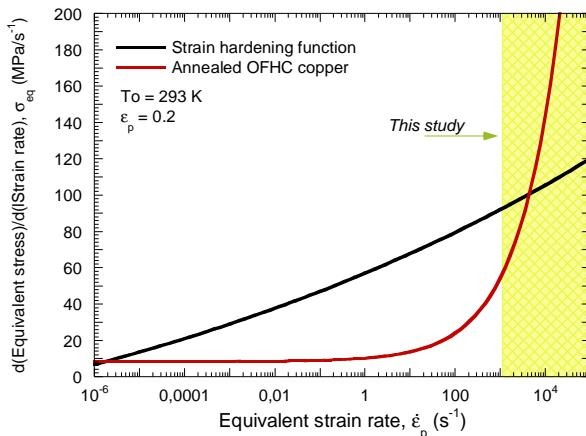
Fig. 3.65. Evolution of the rate sensitivity versus strain rate for the extra strain hardening configuration at room temperature and  $\varepsilon_p=0.2$ . Comparison with annealed OFHC copper.
