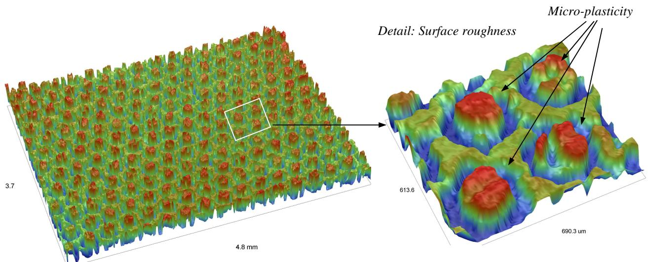
Fig. 5.44. Surface roughness of **TRIP 1000** steel.
