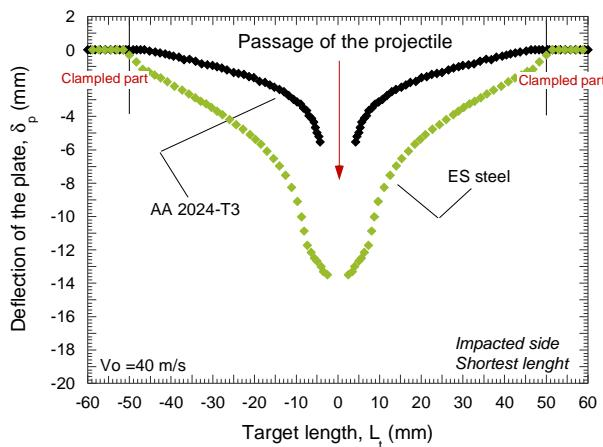
Fig. 4.63. Post-mortem deflection of the target for AA 2024-T3 and steel ES for  $V_0 \approx 40$  m/s.
