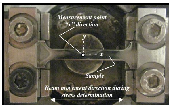
Fig. 5.5. Experimental setup for in situ test (ENSAM/Metz).
