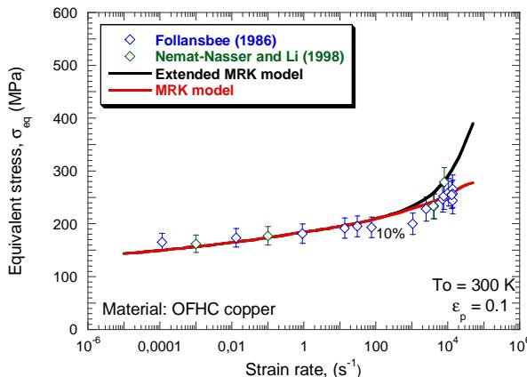
Fig. 2.31. Description of the flow stress evolution as a function of strain rate by original and extended **MRK** models and comparison with experiments at room temperature for  $\varepsilon_p = 0.1$  [Nemat-Nasser and Li 1998].
