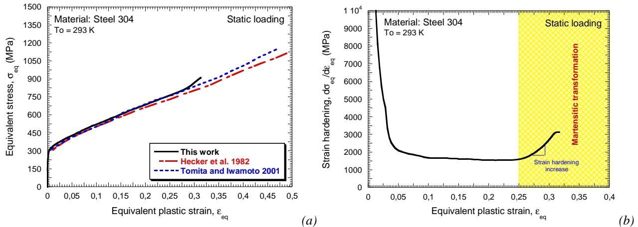
Fig. 5.6. (a) Flow stress evolution versus strain and comparison between our experiments and those reported in [Hecker et al. 1982, Tomita and Iwamoto 2001]. (b) Strain hardening evolution versus strain under static loading at room temperature.
