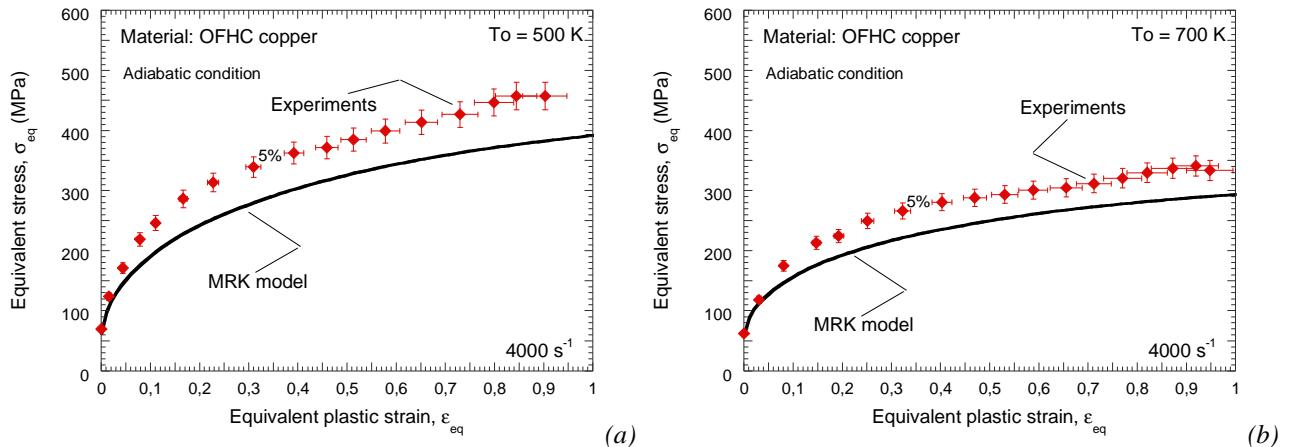
Fig. 2.23. Description of the flow stress evolution as a function of plastic strain by the **MRK** model and comparison with experiments at  $4000 \text{ s}^{-1}$  [Nemat-Nasser and Li 1998]. (a)  $T_0=500 \text{ K}$ , (b)  $T_0=700 \text{ K}$ .
