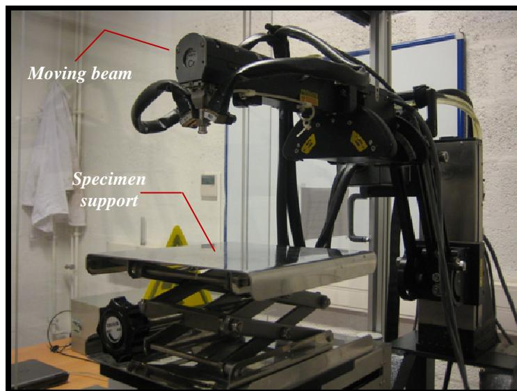
Fig. 5.2. Portable **PROTO** goniometer used for XRD measurement (ENSAM Metz).
