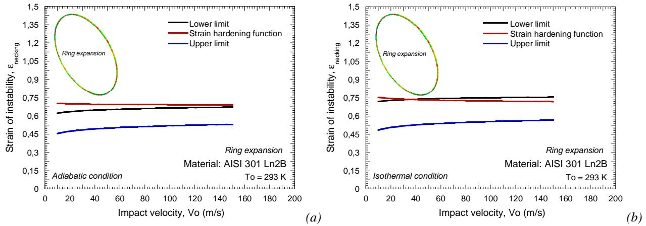
*Fig. 3.69. Strain of instability as a function of impact velocity.
