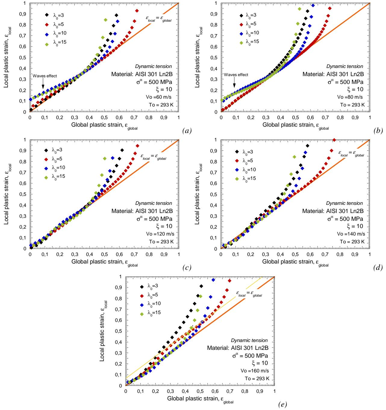
Fig. 3.94. Evolution of the local plastic strain as a function of the global plastic strain for the material configurations analyzed. (a)  $V_0 = 60 \text{ m/s}$ , (b)  $V_0 = 80 \text{ m/s}$ , (c)  $V_0 = 120 \text{ m/s}$ , (d)  $V_0 = 140 \text{ m/s}$ , (e)  $V_0 = 160 \text{ m/s}$ .
