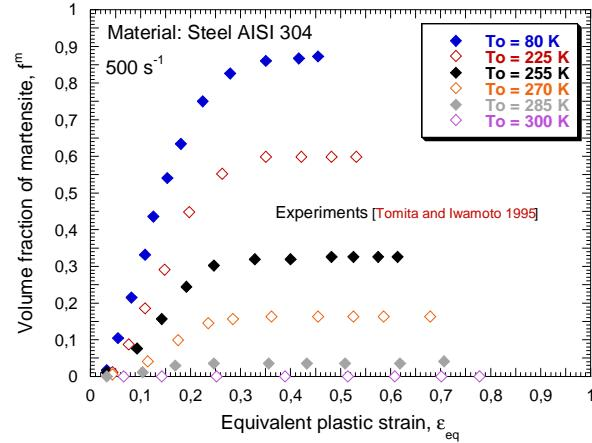
Fig. 2.45. Volume fraction of martensite as a function of plastic deformation for different initial temperatures.
