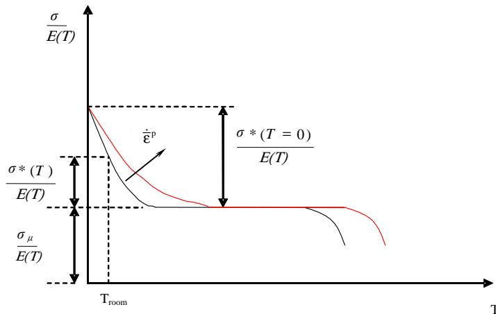
Fig. 2.1. Decomposition of normalized macroscopic stress versus temperature
