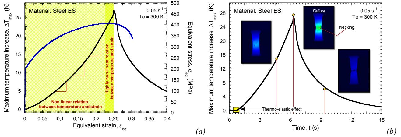
Fig. 4.8. (a) Maximum temperature increase versus plastic strain and flow stress evolution versus plastic strain.
