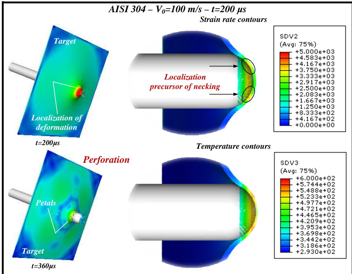
Fig. 5.41. Numerical estimations of strain rate and temperature contours during impact,  $V_0 = 100 \text{ m/s}$
