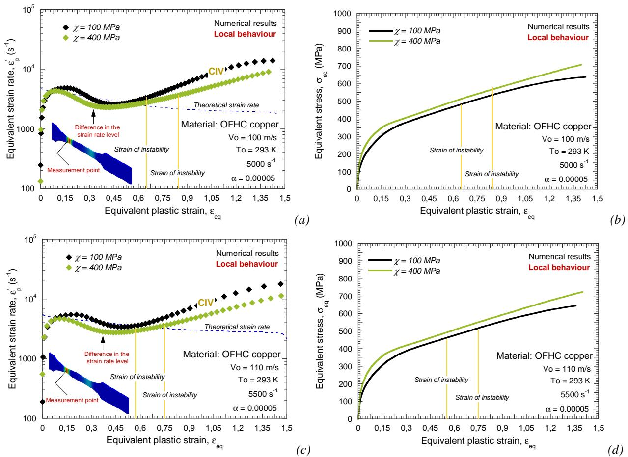
Fig. 3.40. Evolution (a) of strain rate and (b) stress as a function of plastic deformation in the necking zone for  $\chi=100 \text{ MPa}$  and  $\chi=400 \text{ MPa}$  at  $V_0=100 \text{ m/s}$  and  $V_0=110 \text{ m/s}$ .
