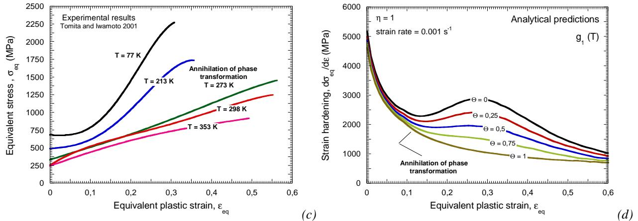
Fig. 2.54. Analytical predictions of the extended RK model (a) in the case of  $g_1(T)$  and (b) in the case of  $g_2(T)$ . (c) Evolution of the flow stress versus the plastic strain for steel AISI 304 [Tomita and Iwamoto 2001]. (d) Description of the strain hardening evolution as a function of plastic strain by the extended RK model for different homologous temperatures.
