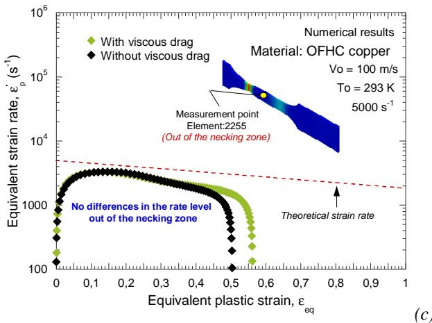
Fig. 3.29. Evolution of strain rate as a function of plastic deformation out of the necking zone for **MRK** and extended **MRK** models. (a)  $V_0=40$  m/s, (b)  $V_0=80$  m/s, (c)  $V_0=100$  m/s.
