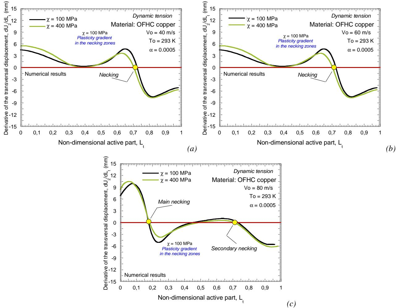
Fig. 3.44. Derivative of the transversal displacement of the active part of the specimen for different values of  $\chi$ .
