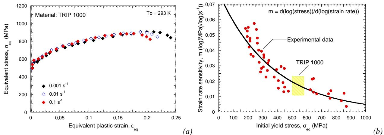
Fig. 5.45. (a) Flow stress of **TRIP 1000** as a function of plastic strain for different loading rates. (b) Evolution of the logarithmic strain rate sensitivity as a function of the initial static yield stress for different steel alloys [Rodríguez-Martínez et al. 2010b].
