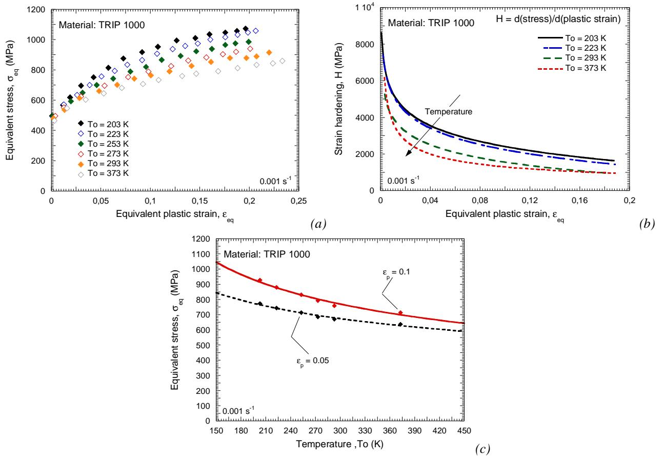
Fig. 5.46. (a) Flow stress of **TRIP 1000** as a function of plastic strain for different initial temperatures. (b) Strain hardening of **TRIP 1000** as a function of plastic strain for different initial temperatures. (c) Evolution of the flow stress as a function of temperature for different plastic strain values.
