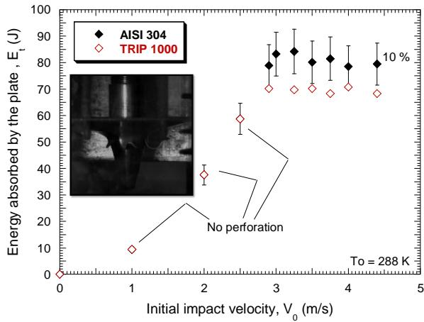
Fig. 5.52. Energy absorbed by the target as a function of the impact velocity for **AISI 304** and **TRIP 1000**.
