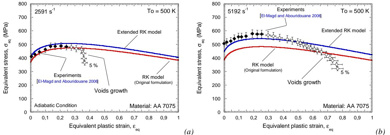
Fig. 2.35. Description of the flow stress evolution versus plastic strain by original and extended **RK** models and comparison with experiments at  $T_0 = 500$  K [El-Magd and Abouridouane 2006]. (a)  $2591 \text{ s}^{-1}$ , (b)  $5192 \text{ s}^{-1}$ .
