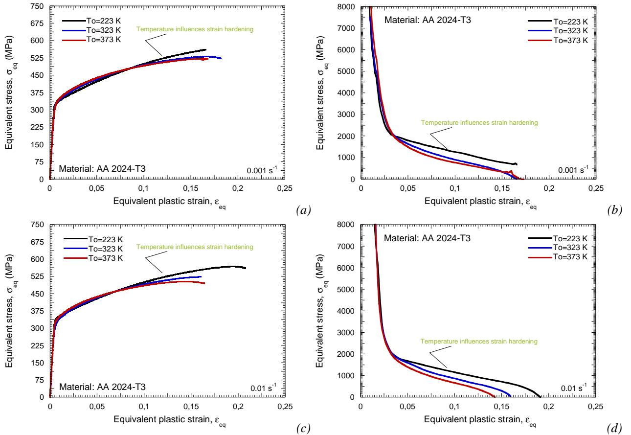
Fig. 4.41. (a) – (c) Flow stress evolution versus plastic strain for different strain rates and initial temperatures.
