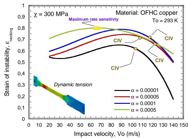
Fig. 3.54. Strain of instability as a function of the impact velocity for different values of  $a$ .
