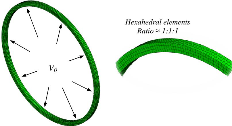
Fig. 3.7. Mesh configuration used in the numerical simulations.
