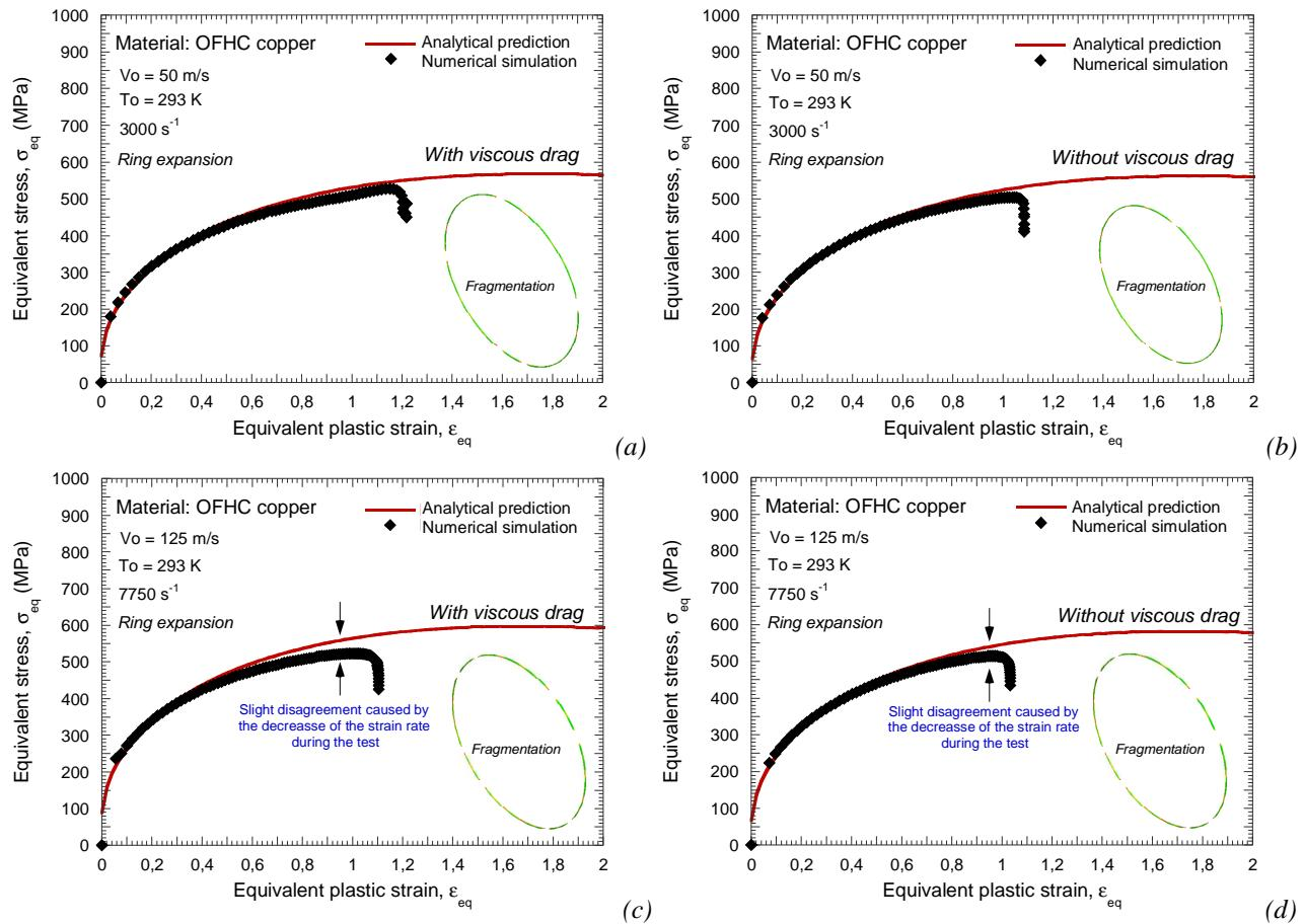
Fig. 3.16. Comparison between numerical results and analytical predictions for MRK and extended MRK models at different impact velocities,  $V_0 = 50 \text{ m/s}$  and  $V_0 = 125 \text{ m/s}$ .
