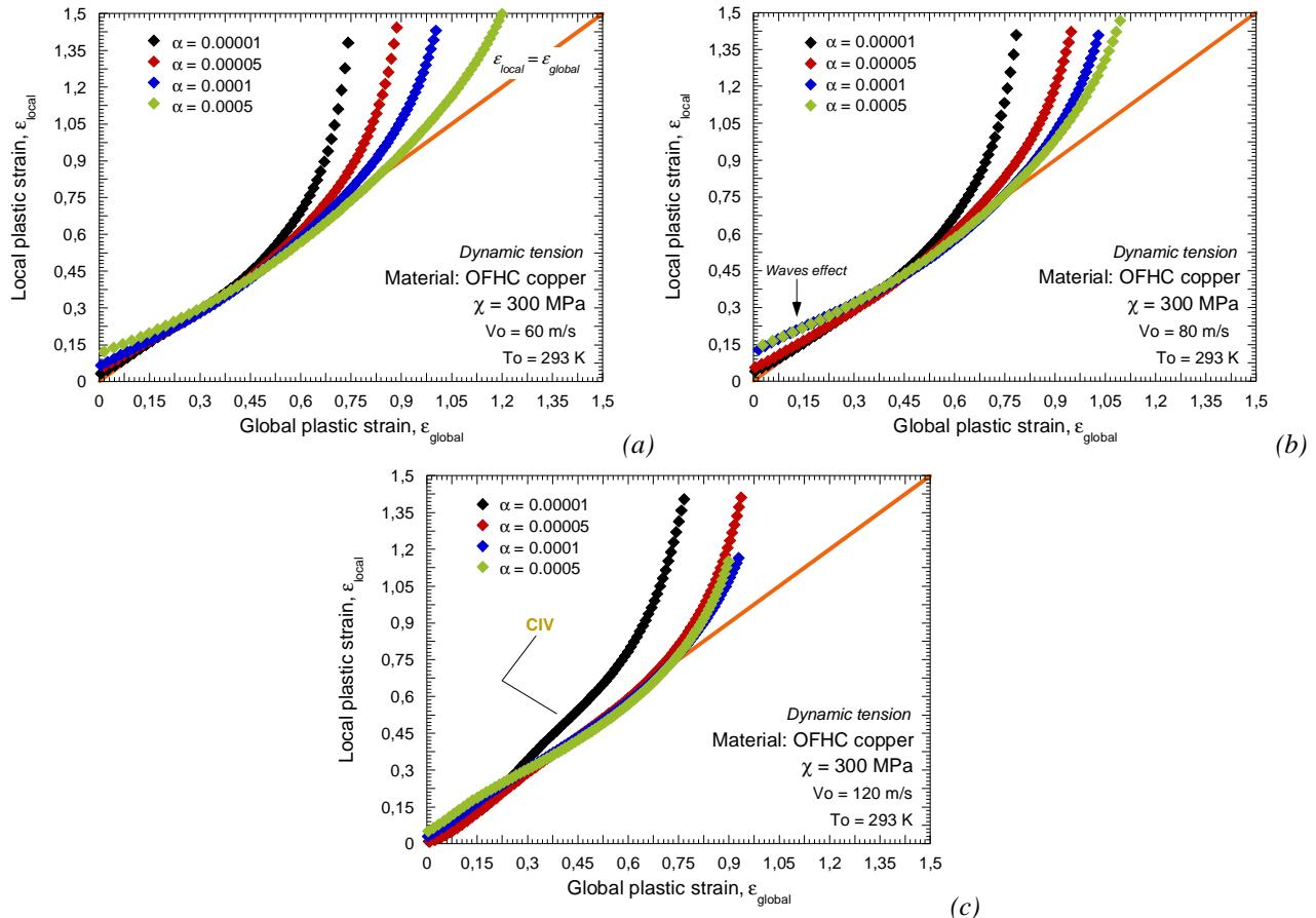
Fig. 3.53. Evolution of the local plastic strain as a function of the global plastic strain for different values of  $\alpha$ .
