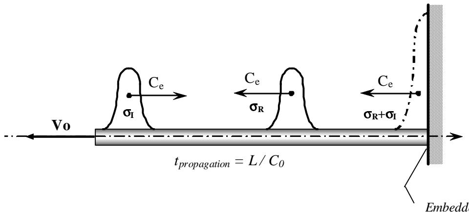
Fig. 3.3. Schematic representation of wave propagation along an elastic bar. Reflection of a longitudinal wave from the fixed end.
