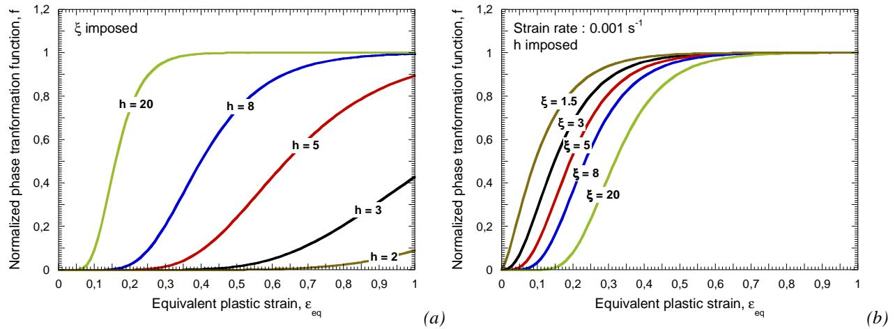
Fig. 2.46. Evolution of phase transformation function  $f(\dot{\bar{\varepsilon}}^p, \bar{\varepsilon}^p)$  as a function of plastic strain, (a) for different values of  $h$ , (b) for different values of  $\xi$ .
