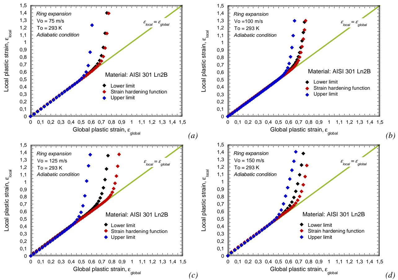
Fig. 3.68. Evolution of the local plastic strain versus the global plastic strain for the configurations analyzed
