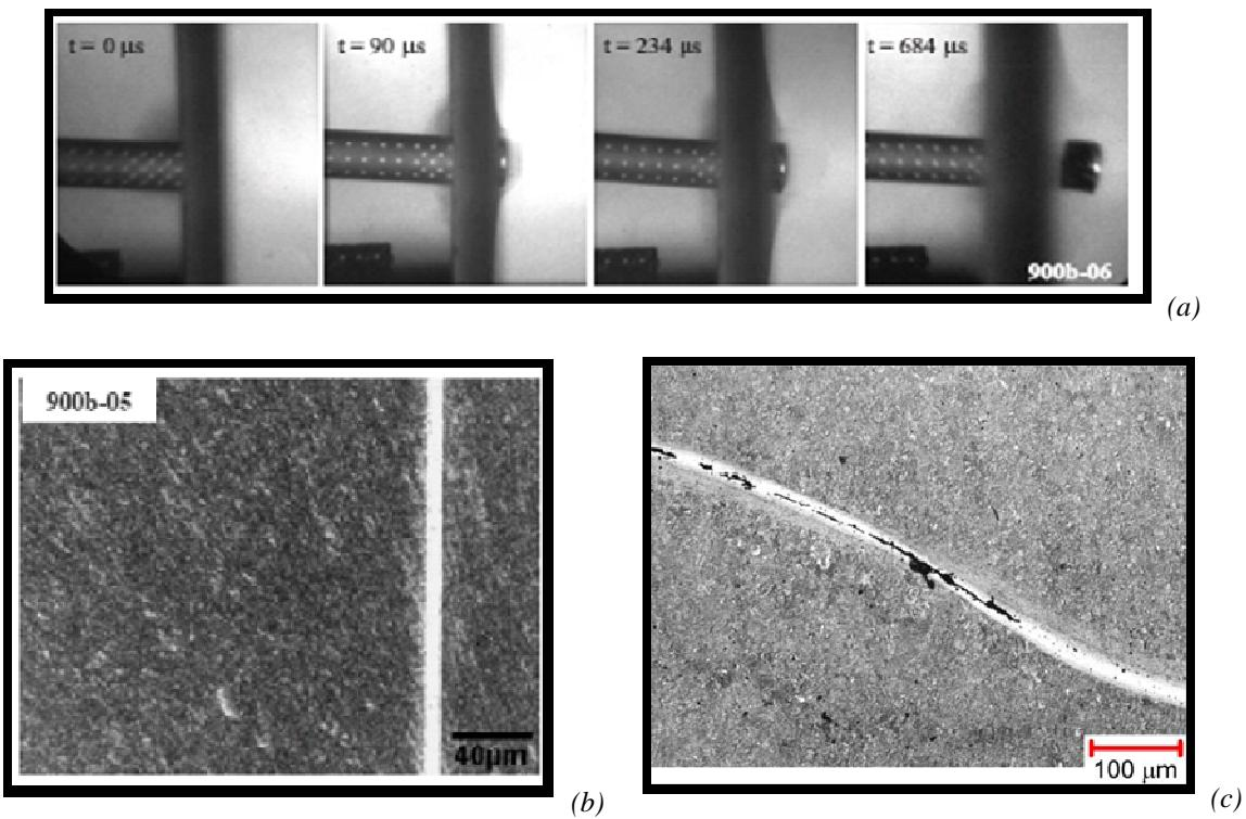
Fig. 1.2. Failure mechanisms taking place under impact. (a) Sequence of images of the perforation process of Weldox 460-E steel plate by a non-deformable blunt projectile with flat faces [Dey et al. 2004]. (b) Adiabatic shear band in a plate of steel Weldox 460-E impacted by a non-deformable blunt projectile with flat faces [Dey et al. 2004]. (c) Adiabatic shear band induced by a ballistic impact in a steel plate [Odeshi et al. 2006].
