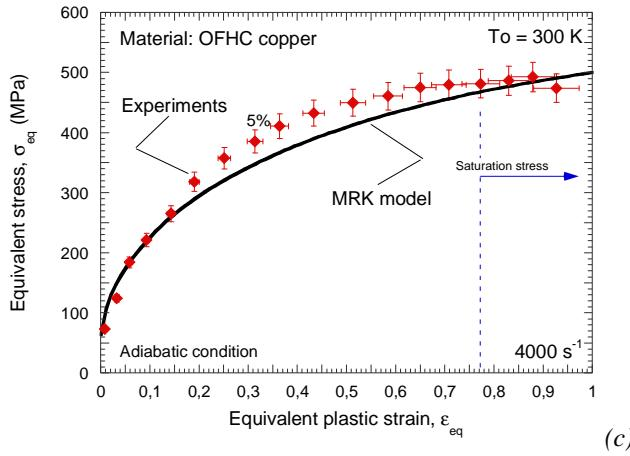
Fig. 2.21. Description of the flow stress evolution as a function of the plastic strain by the **MRK** model and comparison with experiments at room temperature [Nemat-Nasser and Li 1998]. (a)  $0.001\text{ s}^{-1}$ , (b)  $0.1\text{ s}^{-1}$ , (c)  $4000\text{ s}^{-1}$ .
