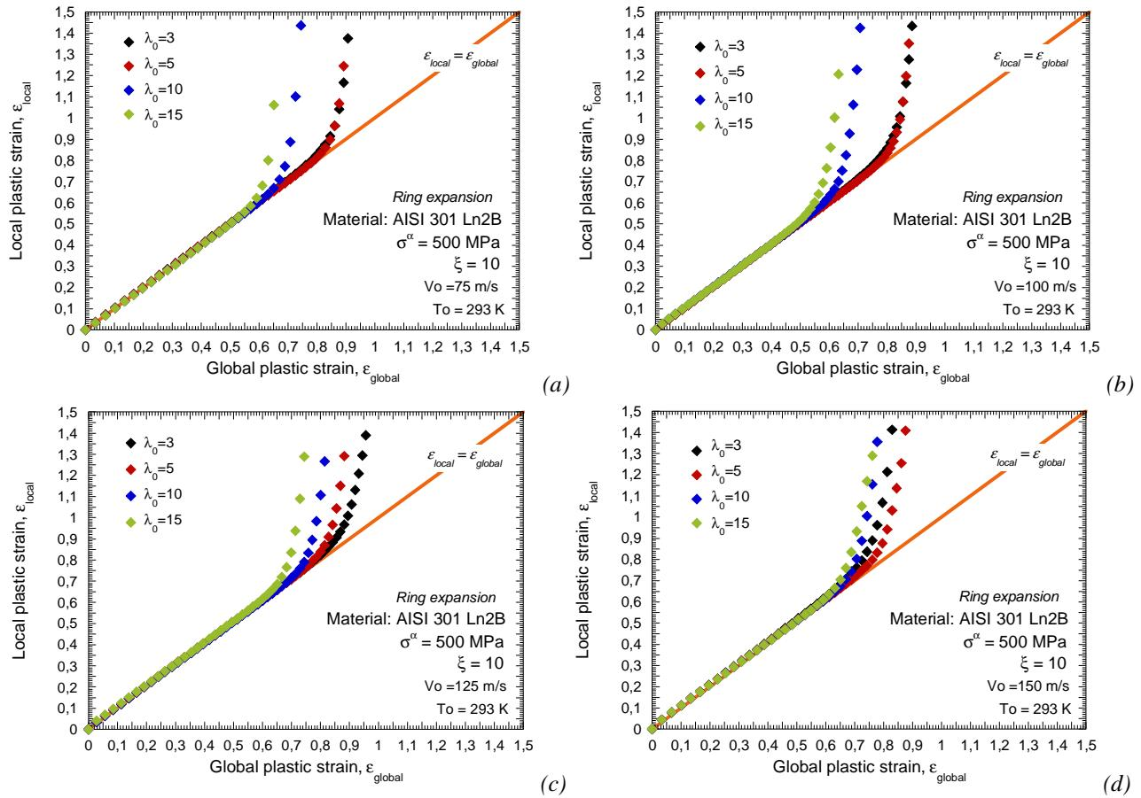
Fig. 3.90. Evolution of the local plastic strain as a function of the global plastic strain for the configurations analyzed
