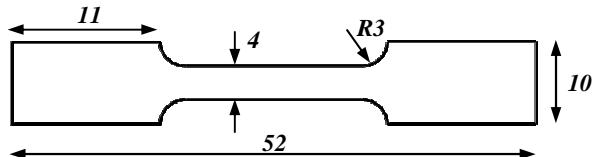
Fig. 5.4. Geometry and dimensions of the in situ tensile specimens.
