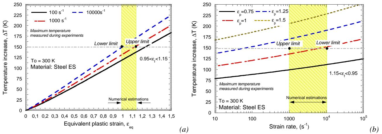
Fig. 4.31. Analytical predictions of the **RK** model for the temperature increase in ES steel. (a) Temperature increase as a function of plastic deformation, (b) temperature increase as a function of strain rate
