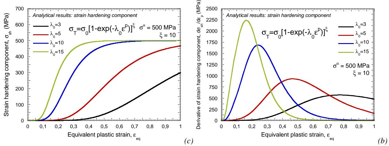
Fig. 3.89. (a) Flow stress predicted by the strain hardening function versus plastic strain for different values of  $\lambda_0$ .
