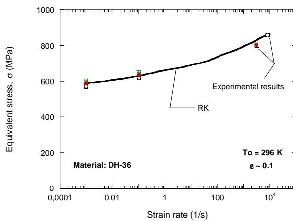
Fig. 2.5. Comparison between modelling (this Thesis) and experiments [Nemat-Nasser and Guo, 2003] for the steel DH-36,  $\dot{\epsilon}_p=0.1$  and room temperature.
