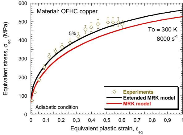
Fig. 2.30. Description of the flow stress evolution as a function of plastic strain by original and extended **MRK** models and comparison with experiments at room temperature for  $8000 \text{ s}^{-1}$  [Nemat-Nasser and Li 1998].
