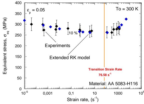
Fig. 2.40. Description of the flow stress evolution as a function of strain rate by the extended RK model and comparison with experiments at room temperature and  $\varepsilon_p=0.05$  [Clausen et al. 2004].
