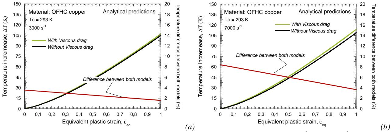
Fig. 3.13. Temperature increase for **MRK** and extended **MRK** models. (a)  $3000 s^{-1}$ , (b)  $7000 s^{-1}$ .
