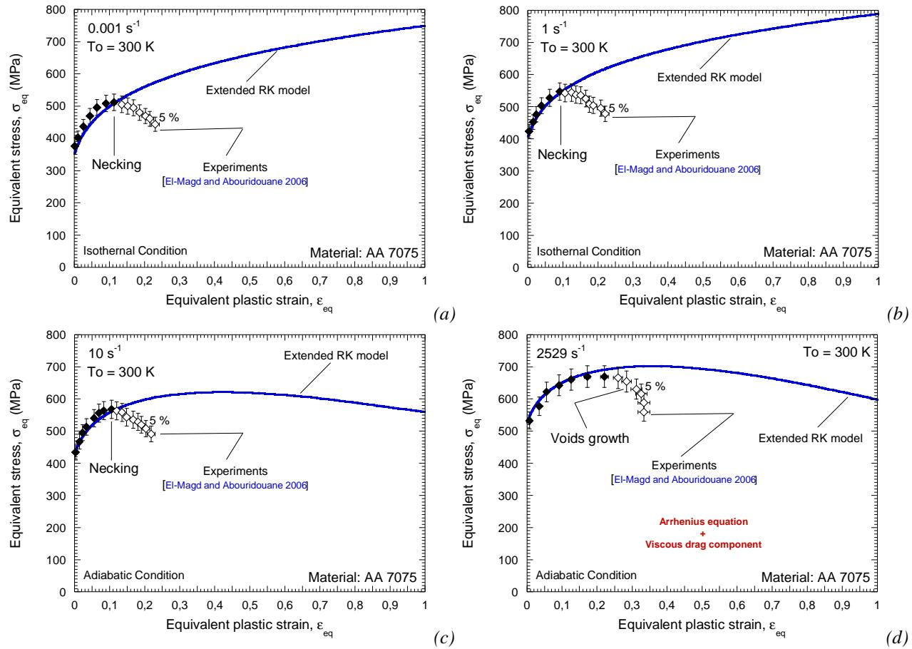
Fig. 2.34. Description of the flow stress evolution versus plastic strain by the extended **RK** model and comparison with experiments at room temperature [El-Magd and Abouridouane 2006]. (a)  $0.001 \text{ s}^{-1}$ , (b)  $1 \text{ s}^{-1}$ , (c)  $10 \text{ s}^{-1}$ , (d)  $2529 \text{ s}^{-1}$ .
