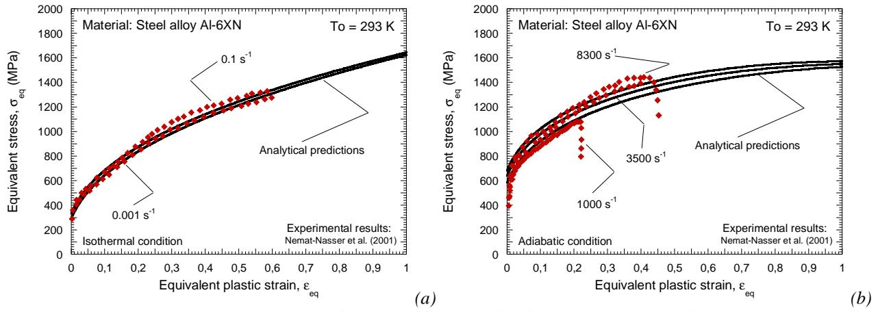
Fig. 2.12. Strain rate effect on the plastic behaviour of the steel alloy AL-6XN, comparison between RK model and experimental results [Nemat-Nasser et al. 2001]. (a) Isothermal conditions of deformation. (b) Adiabatic conditions of deformation.
