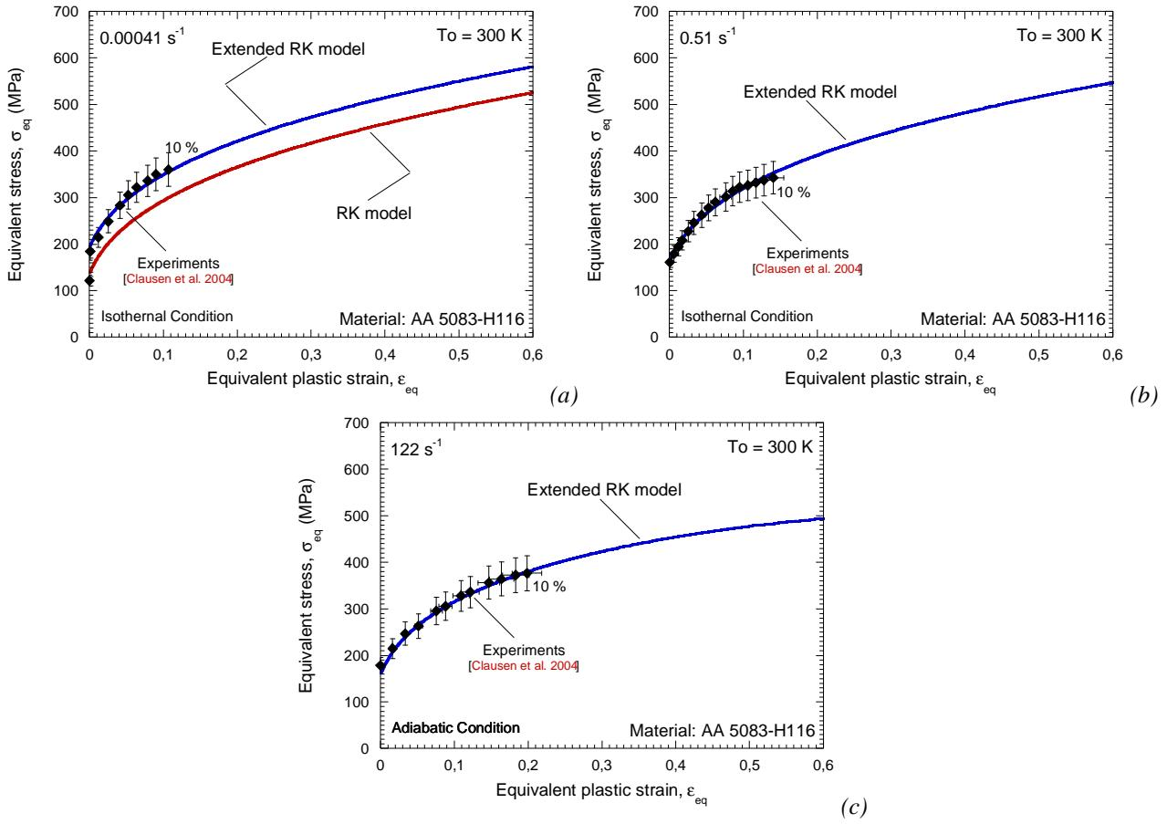
Fig. 2.39. Description of the flow stress evolution as a function of the plastic strain by the extended RK model and comparison with experiments at room temperature [Clausen et al. 2004]. (a)  $0.00041 \text{ s}^{-1}$ , (b)  $0.51 \text{ s}^{-1}$ , (c)  $122 \text{ s}^{-1}$ .
