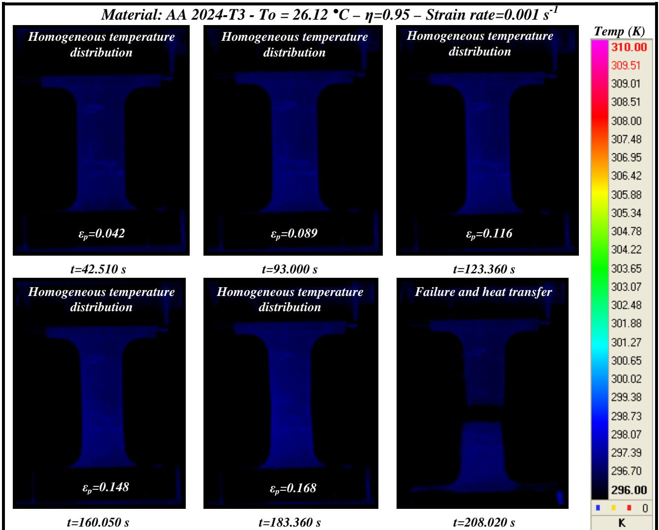
Fig. 4.38. Temperature contours during loading. Picture resolution 320×256 pixels.
