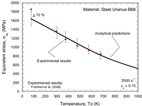
Fig. 2.18. Flow stress evolution as a function of the initial temperature. Comparison between analytical predictions and experiments [Frechard et al. 2008]. Strain rate  $0.1 \text{ s}^{-1}$  and  $\epsilon_p = 0.15$ .
