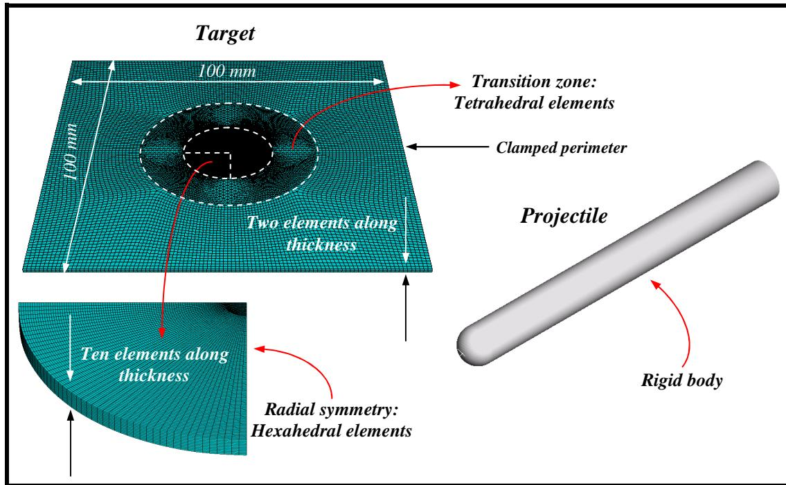
Fig. 4.28. Numerical configuration used in the simulations.
