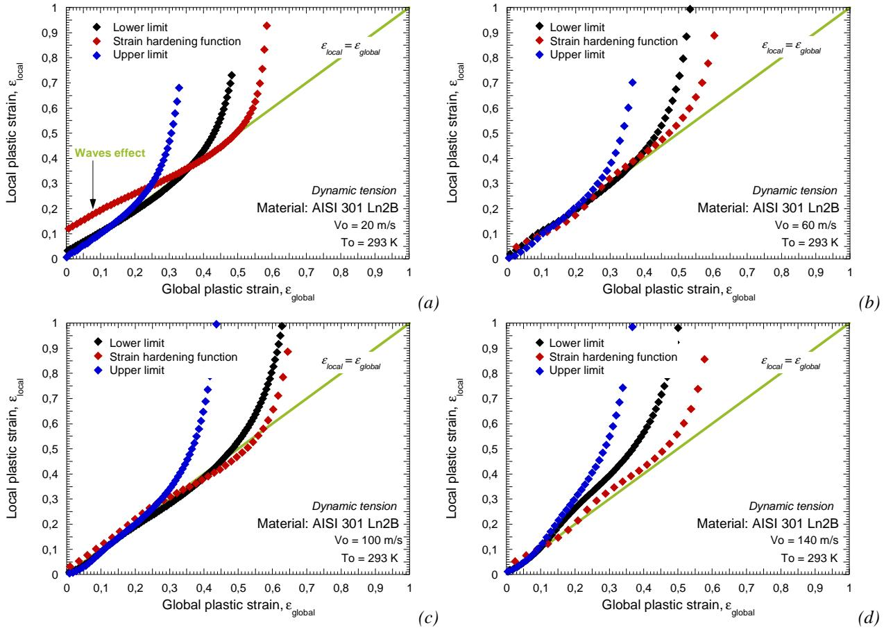
Fig. 3.72. Evolution of the local plastic strain versus the global plastic strain for the three configurations analyzed
