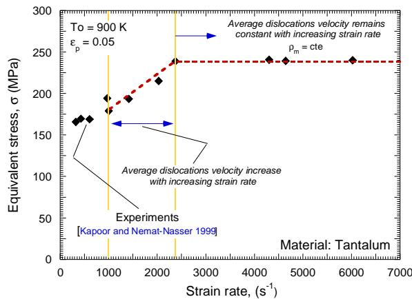
Fig. 2.26. Experimental data of the flow stress evolution as a function of strain rate for Tantalum for  $\epsilon_p=0.05$  at  $T_0=900\text{K}$ . Definition of the stages of the viscous drag process [Kapoor and Nemat-Nasser 1999].
