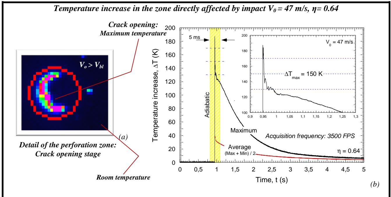
Fig. 4.26. Temperature increase in the impact zone.  $V_0 = 47 \text{ m/s}$ .
