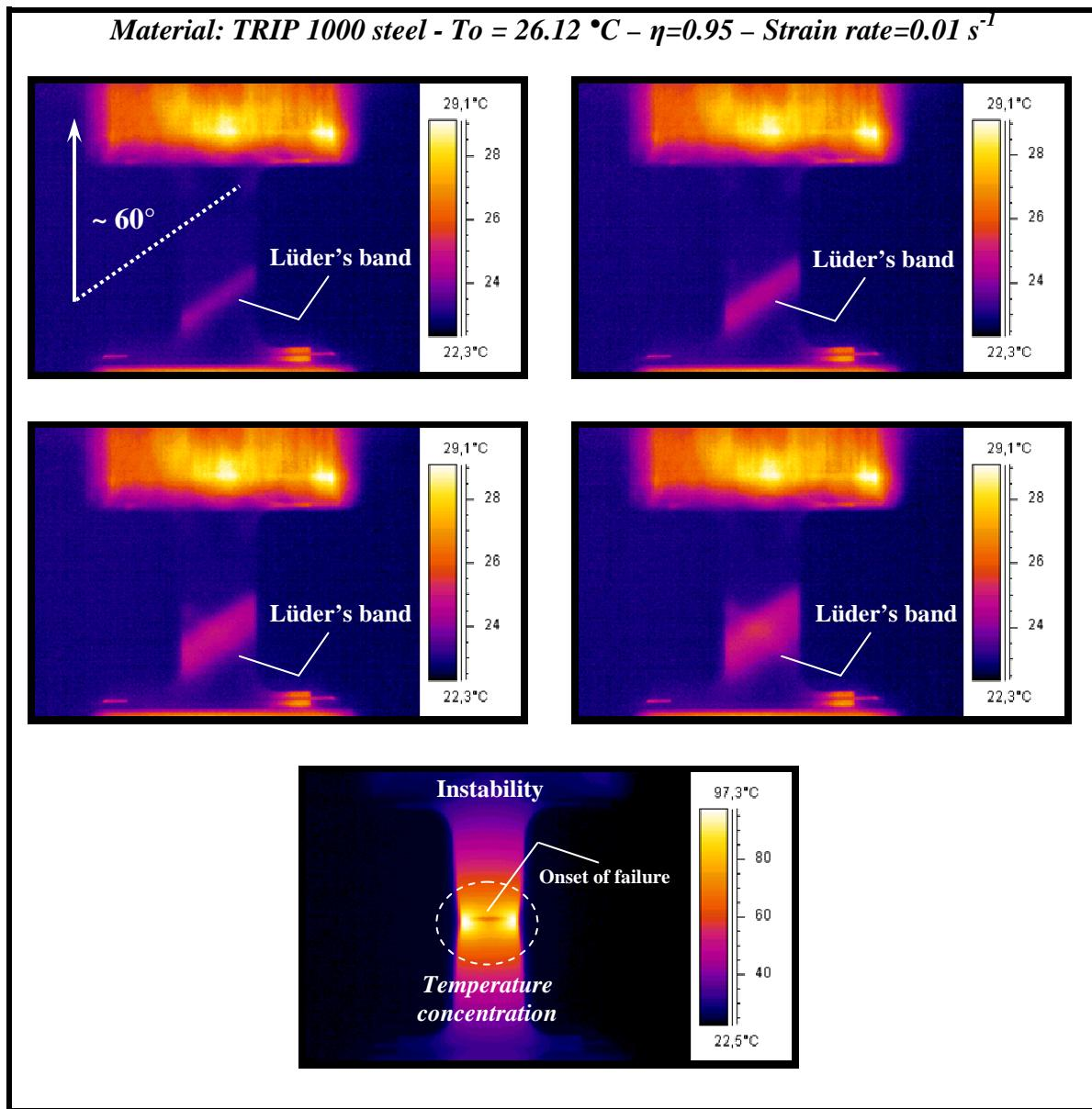
Fig. 5.47. Temperature contours during loading [Rusinek and Klepaczko 2009].
