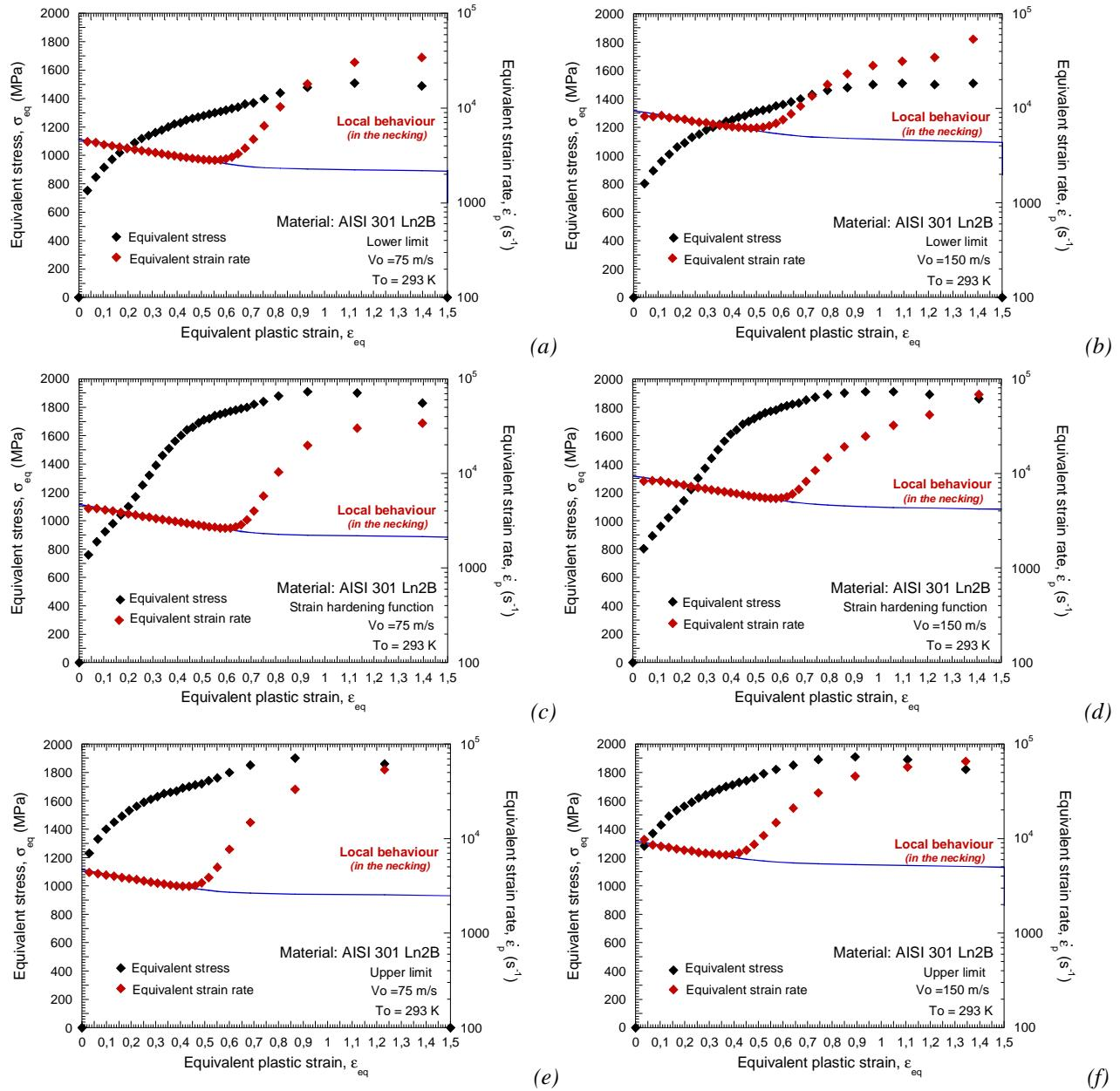
Fig. 3.71. Evolution of the stress and strain rate in the necking as a function of plastic strain for the three material configurations considered and different impact velocities.
