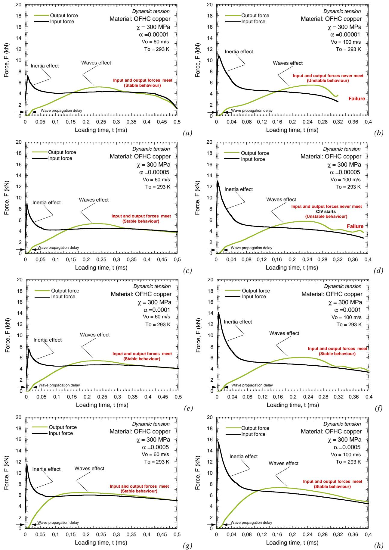
Fig. 3.55. Output and input forces for different values of  $\alpha$  and two impact velocities,  $V_0=60 \text{ m/s}$  and  $V_0=100 \text{ m/s}$ .
