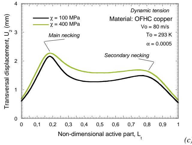
Fig. 3.43. Transversal displacement of the active part of the specimen for different values of  $\chi$ .
