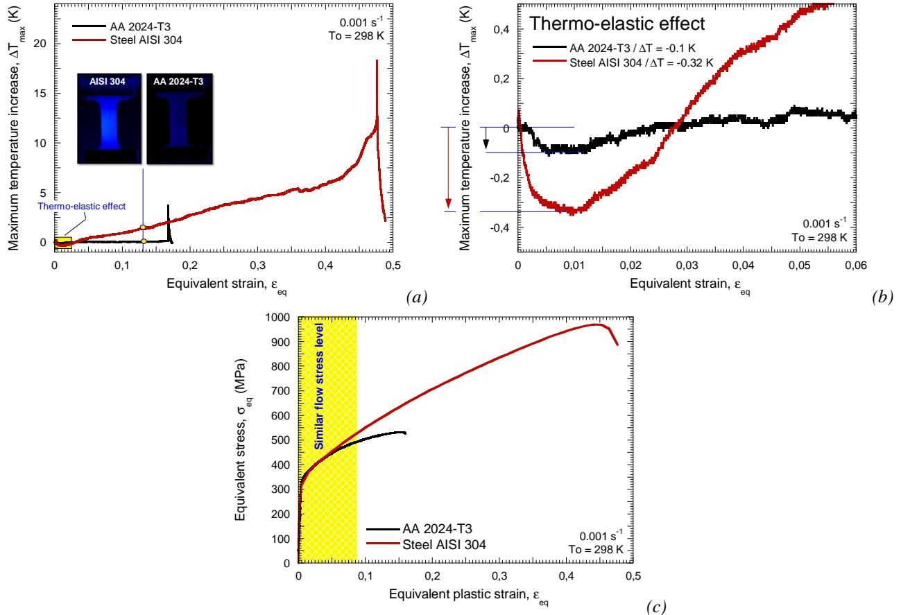
Fig. 5.11. (a) Temperature variation as a function of strain for AA 2024-T3 and steel AISI 304. (b) Temperature decrease due to thermo elasticity. (c) Flow stress evolution as a function of plastic strain for AA 2024-T3 and steel AISI 304 under static loading at room temperature.
