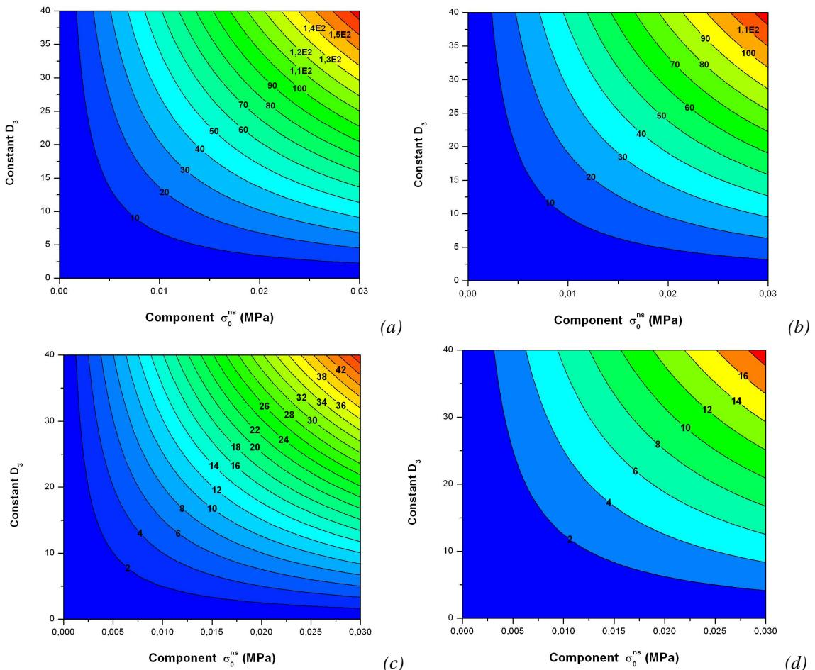
Fig. 2.37. Evolution of the **NSRS** stress component as a function of  $\sigma_0^{ns}$  and  $D_3$  for different strain rate levels at room temperature. (a)  $0.001 s^{-1}$ , (b)  $0.01 s^{-1}$ , (c)  $1 s^{-1}$ , (d)  $10 s^{-1}$ .
