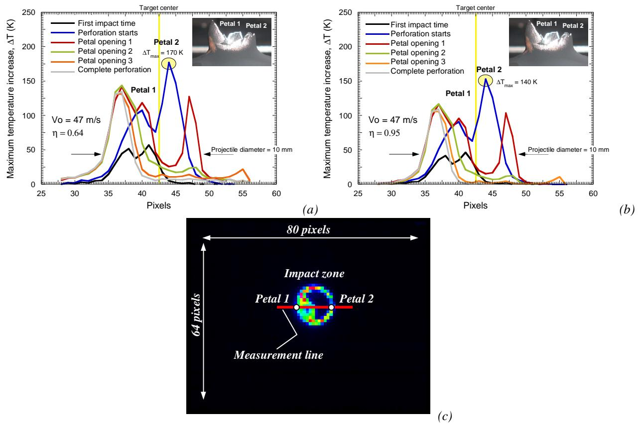
Fig. 4.25. Maximum temperature increase in the impact zone at  $V_0 = 47$  m/s (a)  $\eta=0.64$  and (b)  $\eta=0.95$ .
