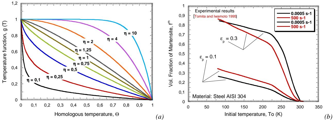
Fig. 2.48. (a) Evolution of the temperature function  $g_1(T)$  as a function of the initial temperature for different values of  $\eta$ .
