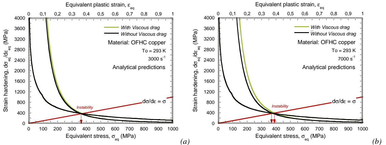
Fig. 3.14. Strain hardening evolution versus plastic strain and versus flow stress for MRK and extended MRK models.
