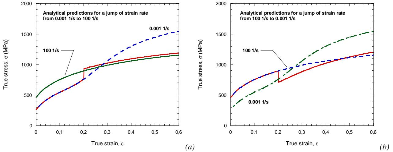
Fig. 2.53. Analytical predictions of the extended RK model in the case of (a) positive and (b) negative jump of strain rate for  $g(T) = 1$ .
