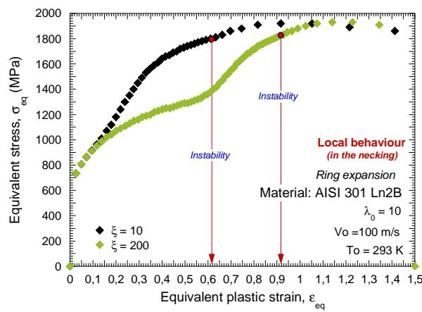
Fig. 3.81. Evolution of stress versus plastic strain in the necking for different values of  $\xi$  at  $V_0=100$  m/s.
