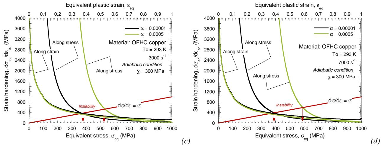
Fig. 3.46. (a)-(b) Flow stress evolution as a function of the plastic strain for different values of  $\alpha$ . (c)-(d) Strain hardening evolution as a function of plastic strain and stress for different values of  $\alpha$ .
