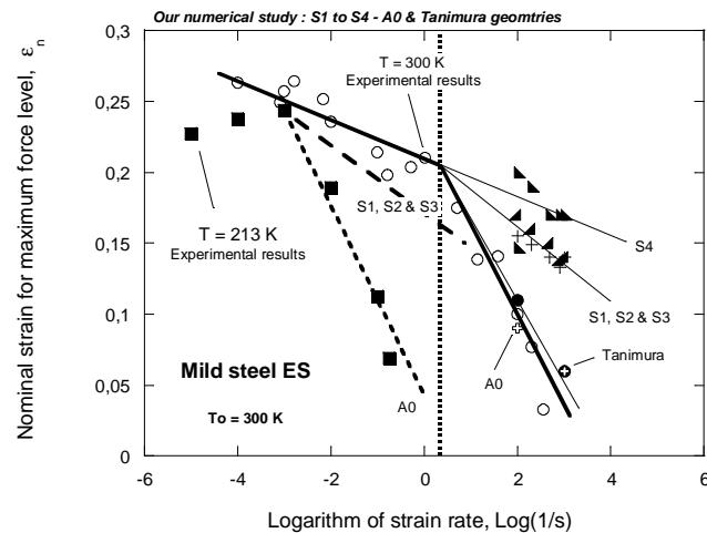
Fig. 4.2. Evolution of failure strain versus strain rate at different initial temperatures [Rusinek et al. 2005].
