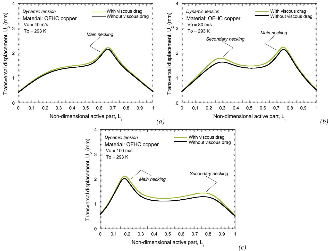
Fig. 3.28. Transversal displacement of the active part of the specimen for **MRK** and extended **MRK** models.
