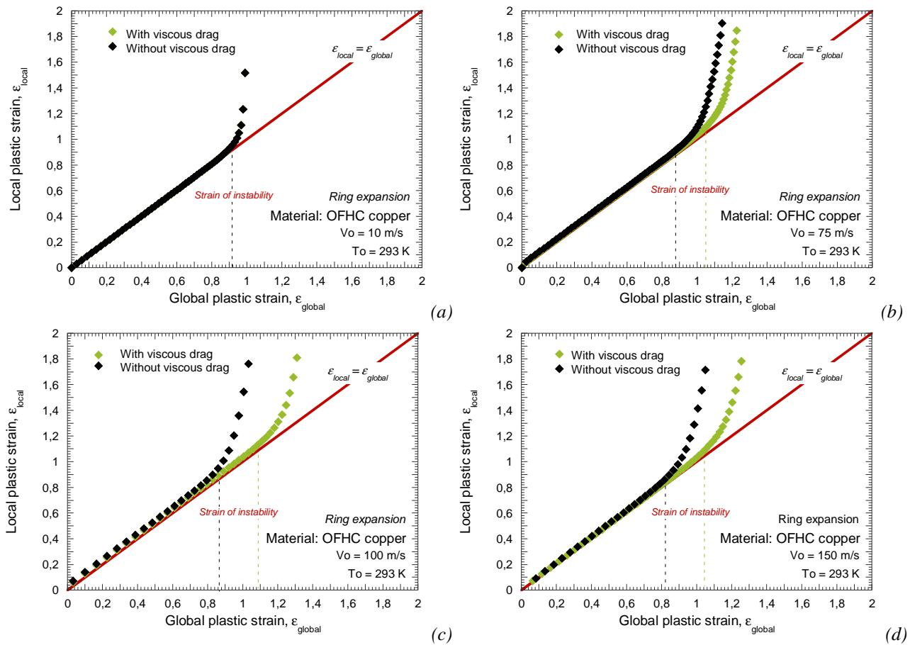
Fig. 3.19. Evolution of the local plastic strain as a function of the global plastic strain for **MRK** and extended **MRK** models. (a)  $V_0 = 10 \text{ m/s}$ , (b)  $V_0 = 75 \text{ m/s}$ , (c)  $V_0 = 100 \text{ m/s}$ , (d)  $V_0 = 150 \text{ m/s}$ .
