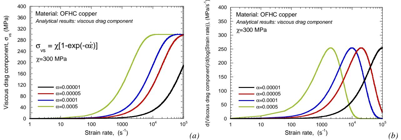
Fig. 3.45. (a) Viscous drag stress component as a function of the strain rate for different values of  $\alpha$ . (b) Derivative of the viscous drag stress component as a function of strain rate for different values of  $\alpha$ .
