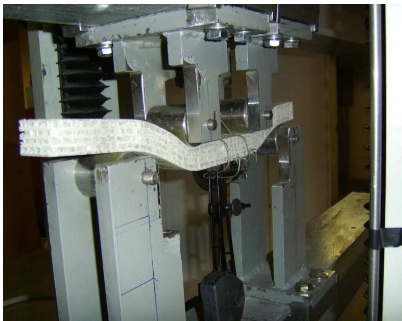
Figure 2.11 Essai de flexion 4 points
