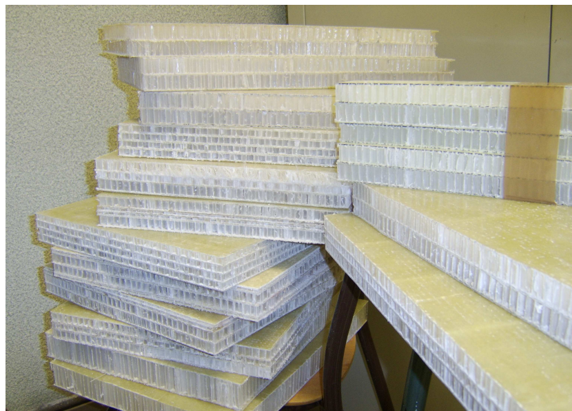
Figure 2.4 Structure sandwich multicouches
