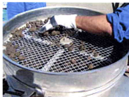
Fig. 11. Soils sampling and sieving.
