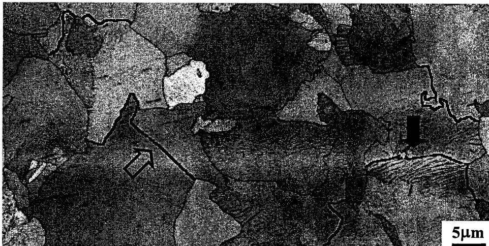
Fig. 7 Detailed locations of \Sigma 3 boundaries. (OIM map of specimens heated at 880°C for 33min and cooled at 10°C/min with the 14 T magnetic field. The magnetic field direction and hot-rolling direction are vertical in this picture. Solid arrow: pearlite boundary; hollow arrow: proeutectoid ferrite boundary. Step size: 0.15 \mu m.
