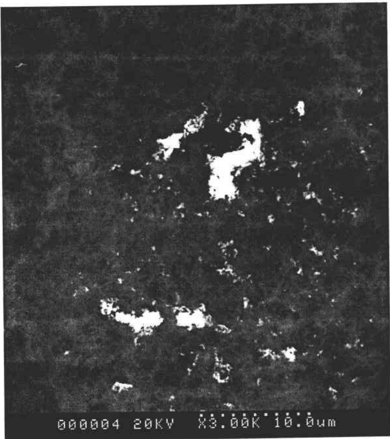
Figure 2: SEM image of the reaction product between dissolved synthetic hydroxyapatite and aqueous lead, at pH adjusted to 3.
