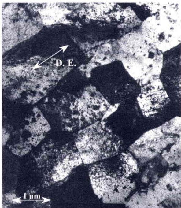
Fig. III.2-1 : Extrusion 1100°C, E.R. = 14 :1.
