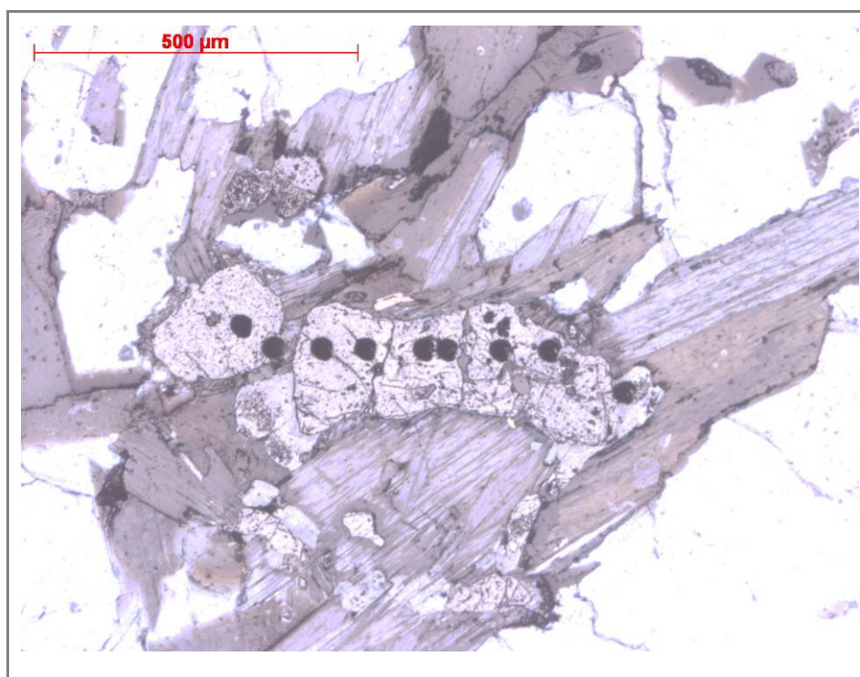
Figure 3.27. Reflected light image of an uraninite from the Namvara ore-showing with the analytical spots created during SIMS U-Pb geochronological dating [sample F134a].
