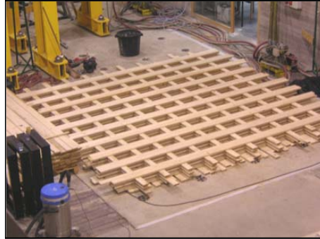
Figure 3. The suspended floor, 4 x 4 m 2 and 216 mm thickness, built of welded spruce slat. M. Properzi et al. (2005) [35].
