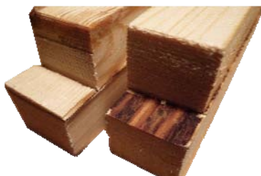
Figure 7. 100% wood failure in samples welded using 1.3 MPa welding pressure, 2.8 s welding time, and 70 s holding time (left). 100% failure in welded interphase in a sample welded using 0.75 MPa welding pressure, 2.8 s welding time, and 70 s holding time
