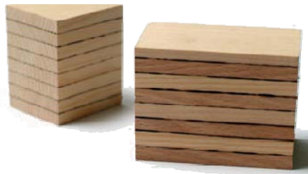
Figure 2. Multilayered wood laminate, built of eight alternating layers of spruce and beech boards; beech shows a darker color. B. Stamm et al. (2005) [34].
