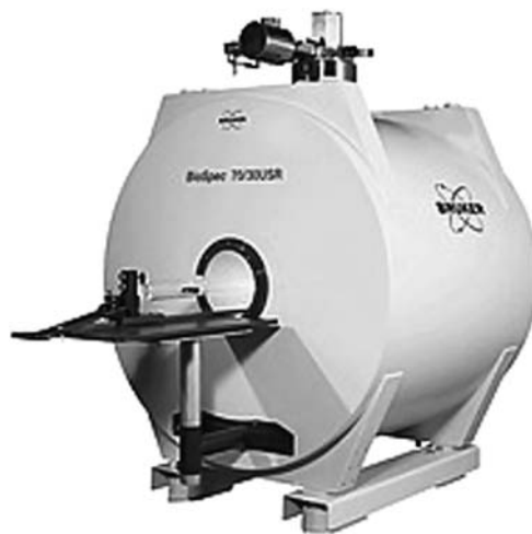
Figure 1. BioSpec, multi purpose high field MRI/MRS research system.
