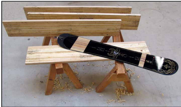
Figure 5. Welded blocks of Populus sp used in the manufacture of snowboard's cores. C. Ganne-Chedeville, (2006) [31].
