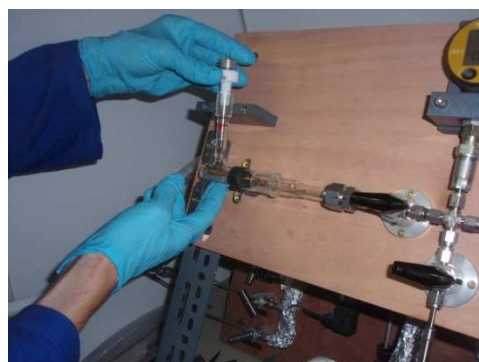
Figure 2.7. Piercing chamber and recovery of the gas phase from the gold capsules after the experiments – see text. The volumes V_1 - V_4 have the following values: V_1 = 30.291 \pm 0.06 \text{ cm}^3 ; V_2 = 0.95 \pm 0.004 \text{ cm}^3 ; V_3 = 1.8276 \pm 0.0035 \text{ cm}^3 ; V_4 = 1.5864 \pm 0.0015 \text{ cm}^3 (designed by Aurélien Randi, G2R, Nancy).
