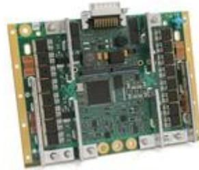
FIG. 2.19 – RP-263XXN0 Solid State Power Controller
