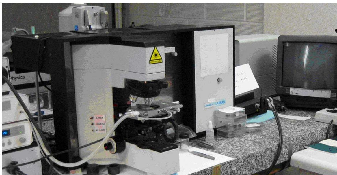
Figure I-8 Photograph of Labram micro-Raman spectrometer (Dilor/Jobin-Yvon/Horiba, USA).
