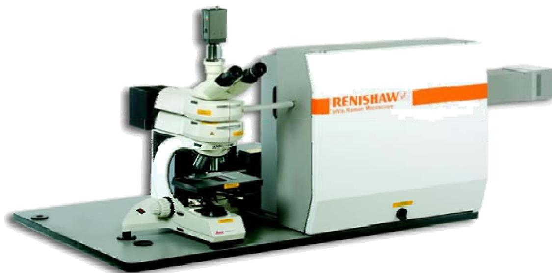
Figure I-9 Photograph of micro-Raman spectrometer (Renishaw, UK)
