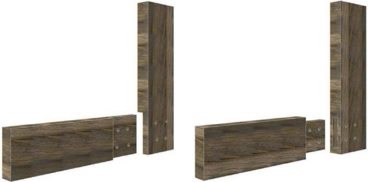
**Parameter A:** Types of Joints: step butt and mortise and tenon.
