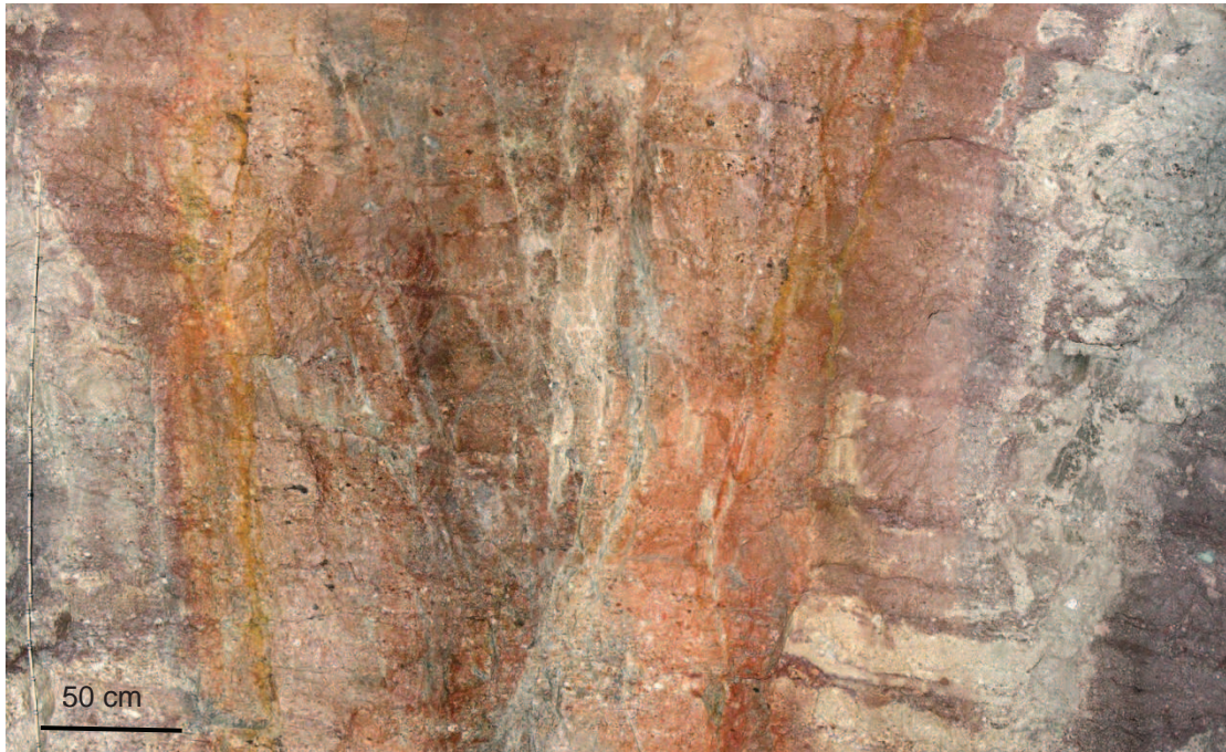
Fig. 2.16. Steeply dipping ore body with disseminated uranium mineralization and relatively wide halo of hematization in tuff-conglomerates. Light-grey – intensively argillized conglomerates, dark brownish-red in the lower right corner – weakly altered conglomerates. Luchisty deposit, horizon +590 m.
