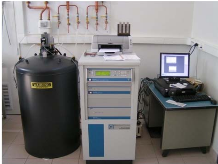
Figure 12 : PPMS-9T (Physical Property Measurements System, Quantum Design)
