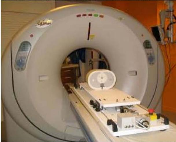
Fig. 3. Dynamic platform placed on the table of the Aquilon 64 CFX multislice CT scanner (Toshiba Medical, Tokyo, Japan).
