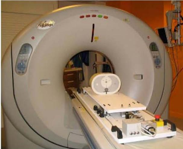
Fig. 2. Dynamic platform placed on the table of the Aquilon 64 CFX multislice CT scanner (Toshiba Medical, Tokyo, Japan)
