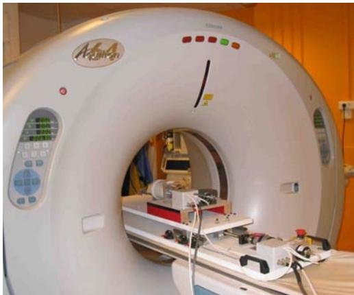
Figure 2. Dynamic Platform, with the original z-axis translation and the added z-axis rotation, placed on the CT table.
