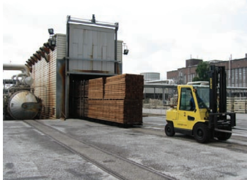
Fig. 1.4 Industrial kiln for the curing stage
