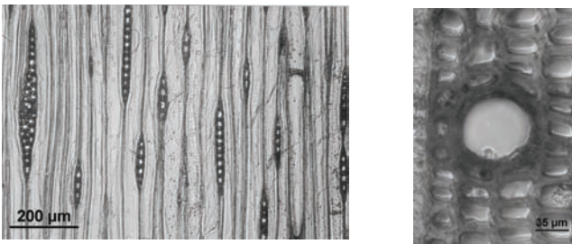
Fig. 2.6a,b Liquid full hydro-thermolysed treated Douglas fir (tangential and cross section), the parenchyma ray cells (a) and epithelial cells of resin canals (b) are not degraded and still intact
