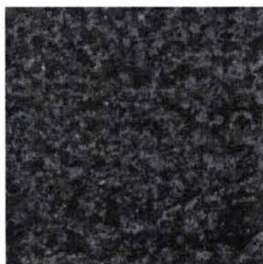
Fig. 3.82 Rusted plate after six hours of exposure in the salt spray chamber.
