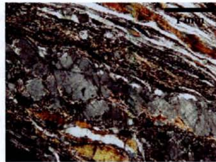
Fig.2.4A - Tessitura cataclastico-milonitica in uno gneiss occhiadino della Sila ( Cataclastic-mylonitic texture in augen gneiss from Sila )
