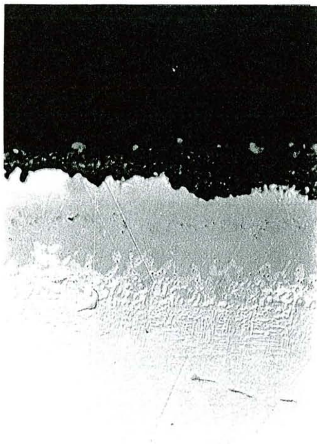
Figure VI-36 : RENE 80 - RT 22 - Corrosion de 506 cycles (x 437)
