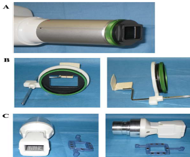
Photo n°16: Collimateurs rectangulaires: A, Type I. B, Type II. C, Type III (Wenjian Z., Kenneth A. and Al., 2009)
