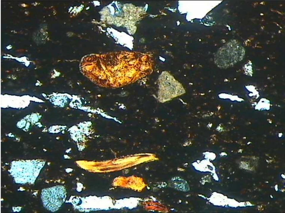
Figure 6 - ASM 5, an intermediate red- buff firing fabric. Orange-yellow grains are of goethite and iron-rich clays from basalt weathering. Limestone grains (e.g. upper right) appear greyish and speckley due to very fine microstructures resulting from thermal decomposition (ppl, magnification x40).
