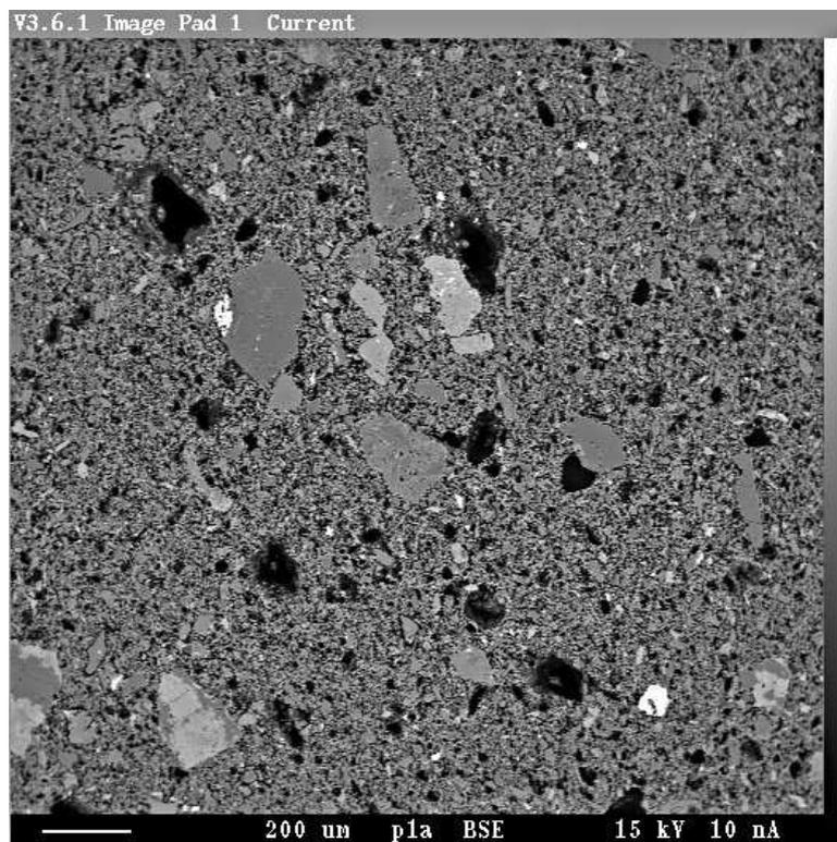
Figure 9 - P1 body showing angular inclusions in a fine-textured calcareous body. Magnification x 50 (scale bar, lower left, is 0.2mm)
