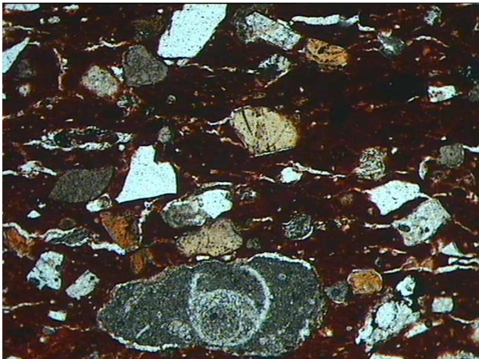
Figure 8 - ASM 10, red-firing with limestone and volcanic inclusions. These are of the same types as for D3 but are slightly coarse. Note the microfossil (foraminifera) still within the original host limestone (micrite). Again the fine sand/silt content of the matrix is relatively low (ppl, magnification x40).
