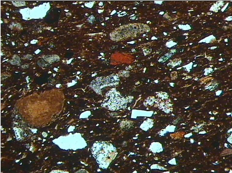
Figure 5 - ASM 7, a buff-firing fabric with limestone and volcanic inclusions. Here there is a high inclusion:matrix ratio (ppl, magnification x40).
