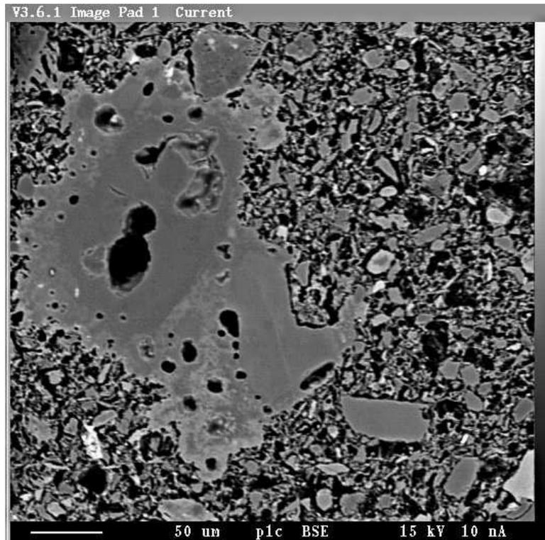
Figure 10 - P1 detail of a fused serpentine inclusion (magnification x 250).
