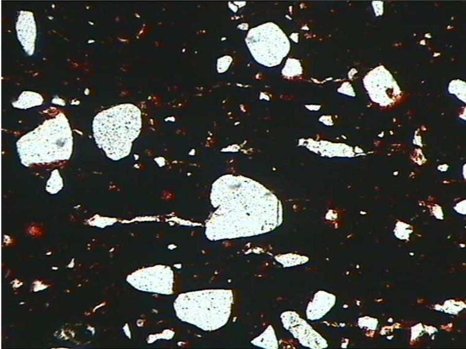
Figure 2 - ASM 12 showing monocrystalline quartz temper in a non-silty matrix (ppl, magnification x40).
