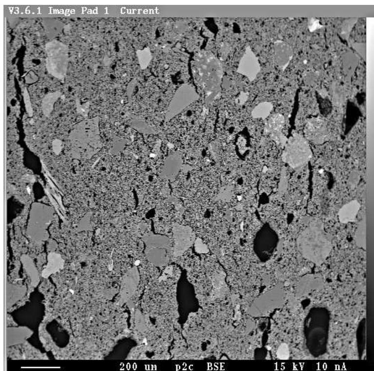
Figure 11 - P2 body - the inclusion types are similar to those of the P1 body (figure 1 ) but are more abundant (magnification x 50)
