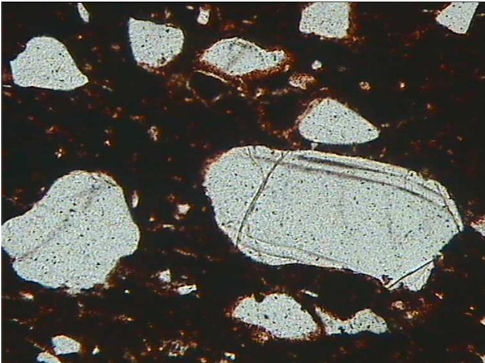
Figure 3 - Detail of ASM 12 showing slightly curved growth lines parallel to the long-axis of the larger quartz grain. These quartz grains are interpreted as being derived from a vein or weak sedimentary quartzite source, and were added as temper to a reddish clay derived (at least in part) from the weathering of a basalt (ppl, magnification x100).
