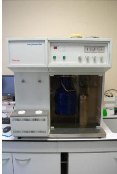
**Figure III. 20 : Appareil Sorptomatic 1990**
