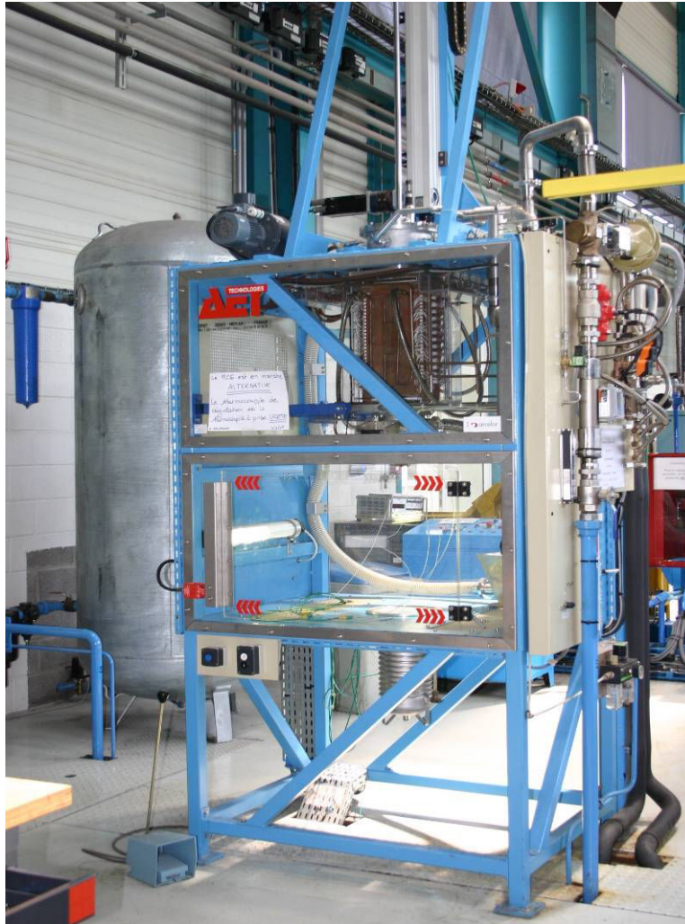
Figure A1.5. AET continuous annealing simulator.
