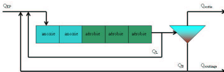
FIG. C.1 – Structure du benchmark BSM1
