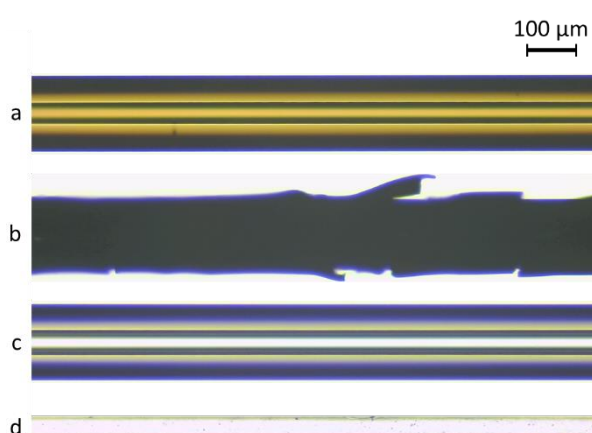
Figure A1.2: Capillaries of 30 \mu\text{m} ID and 150 \mu\text{m} OD (a) with the polyacrylamide sheath, (b) with the burned polyacrylamide sheath, (c) without the polyacrylamide sheath, and (d) after complete etching. All were observed under a microscope.
