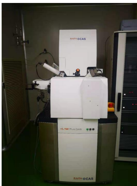
Figure 2. 8 E-Line Plus electron beam lithography machine.
