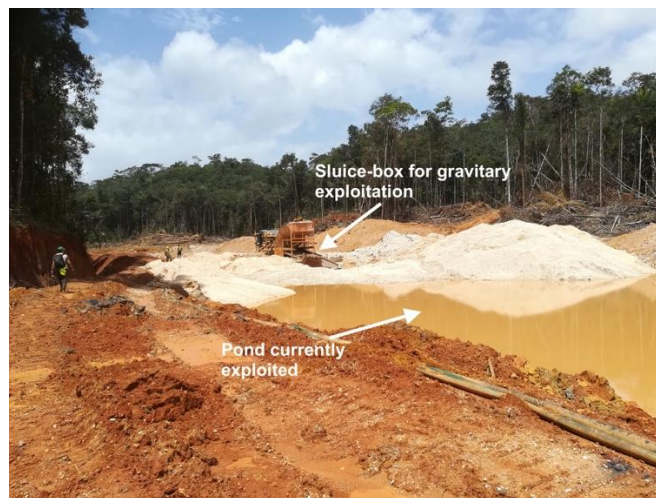
A mining dam system in a ASM project type. The pond currently exploited and the sluice-boxes used for gravitary exploitation
