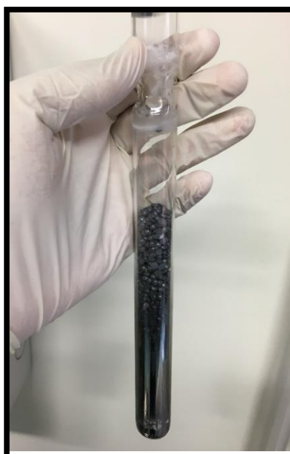
Figure 3.10: Sealed quartz tube with Tellurium to be placed in the vertical rocking furnace.
