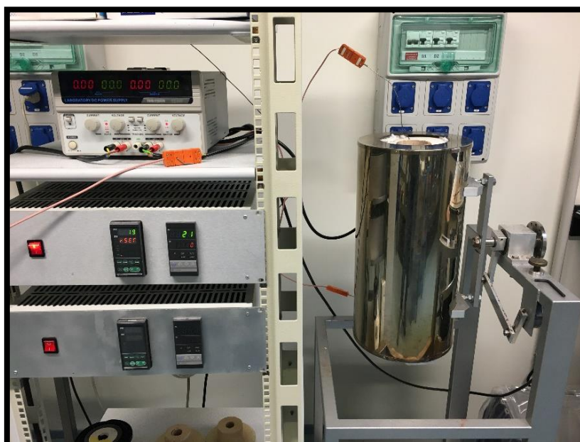
Figure 3.11: High-temperature vertical rocking furnace.
