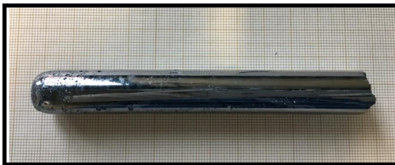
Figure 4.11: Prepared polycrystalline InTe ingot before introduction in the carefully-designed V-shaped-end silica tube for Bridgman-Stockbarger process.
