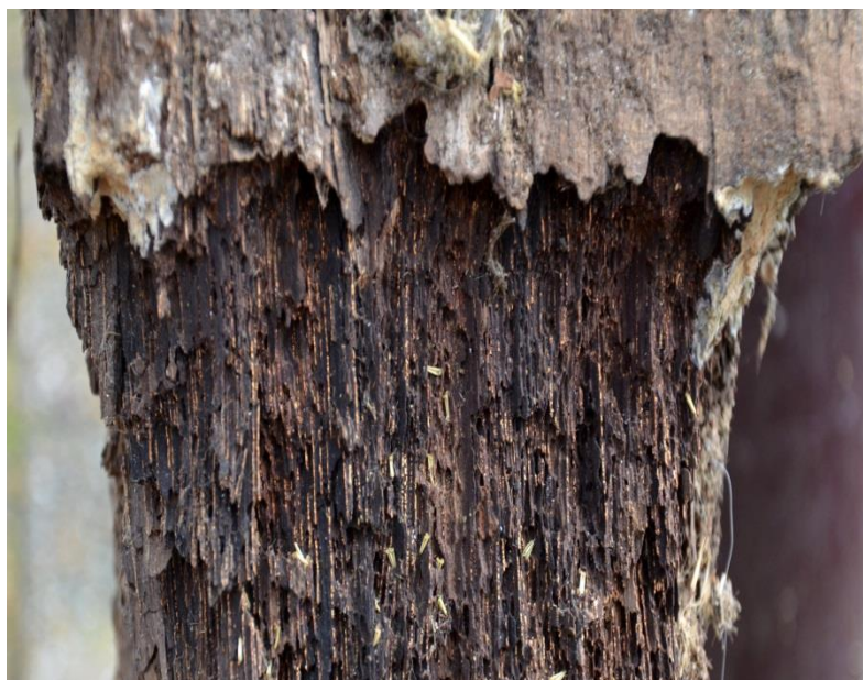
Fig 17: Wood degraded by fungi (Wikimedia commons, 2019)
