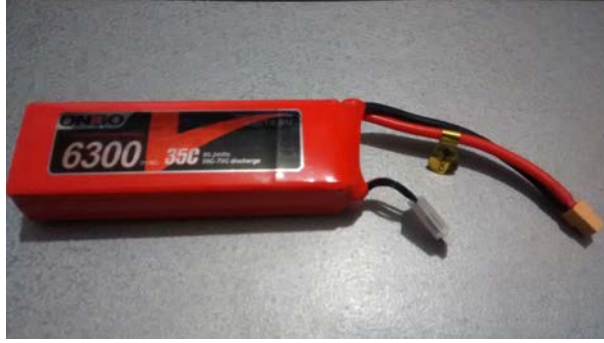
Figure 3.8: Typically Li-Po battery used in multirotor UAV applications.
