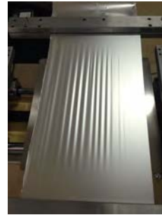
Figure 1.2: Instability in metal film under uni-axial tension
