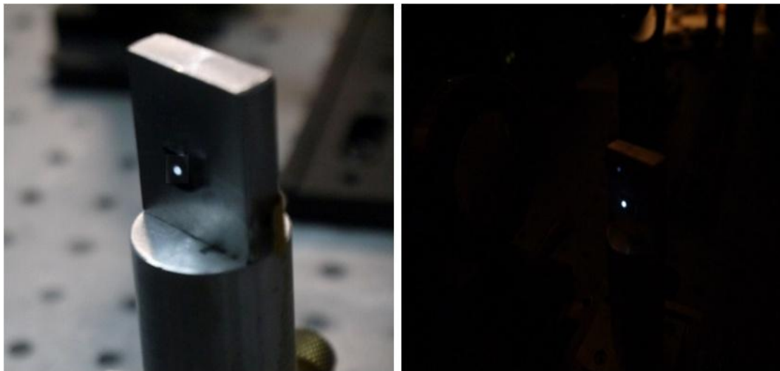
Fig (4.31): White emission photos with bright and dark background from 1% Ce-doped Al(O)N of 7% oxygen and 5 \mu\text{m} thickness excited by a 325 nm laser
