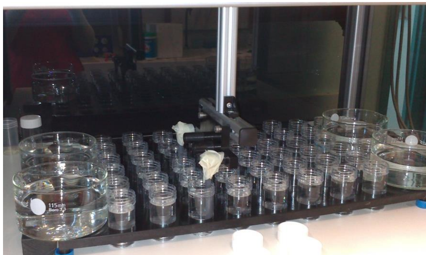
Figure 2.36. Automated dip coating (Dipping robot, Riegler and Kirstien, GmbH, Berlin, Germany)
