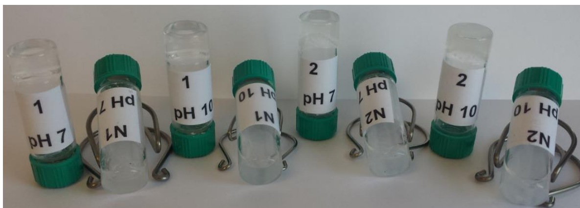
Figure 7.12. Effect of insertion of aza-amino acid on the MGCs. Hydrogels obtained from compounds 7a' (vial 1), and 7b' (vial 2) versus viscous solution from the corresponding peptides without aza-moiety, vial N1 = Fmoc-FFA, and vial N2 = Fmoc- D -FFA; (1.0 wt%, pH 7.0 and 10.0).
