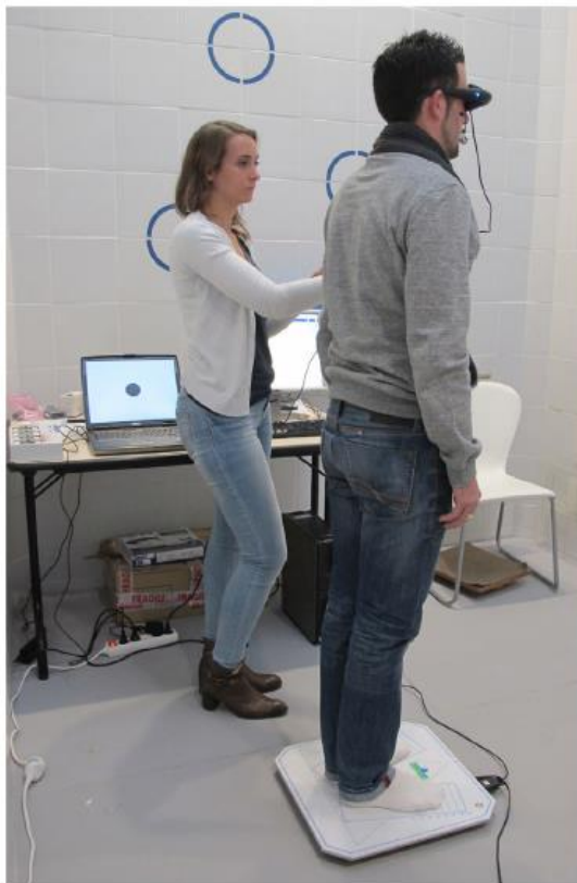
FIGURE 2 | Postural control analysis on a posturography platform (Medicapture, Balma, France). Virtual reality goggles (RM Ingénierie, Rodez, France).
