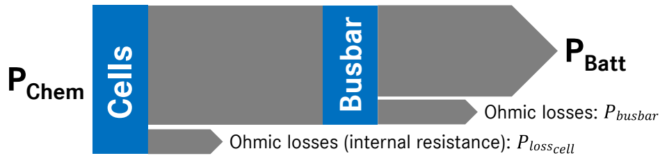
Figure 97: Sankey diagram of the battery as considered in this work
