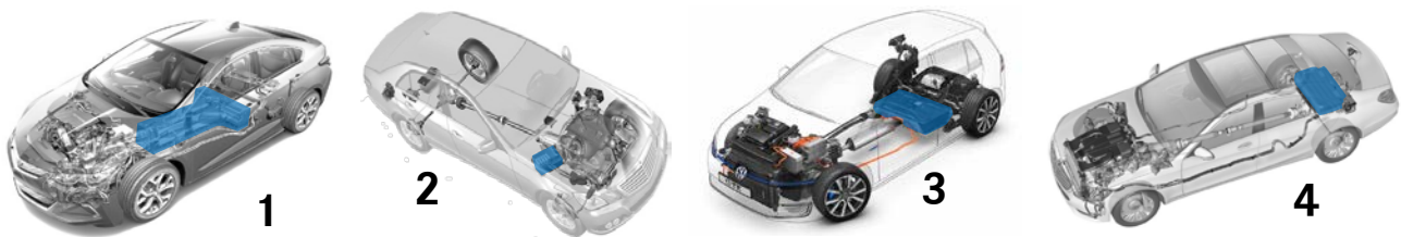
Figure 8: Integration of battery in hybrid vehicles [18], [23], [26] and [19]
