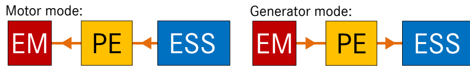
Figure 4: Motor mode (left) and generator mode (right) in electric drives adapted from [9]
