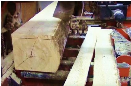
Figure 107. Splitting of a log into boards with a band saw. (LindasawmillCinema, 2016)
