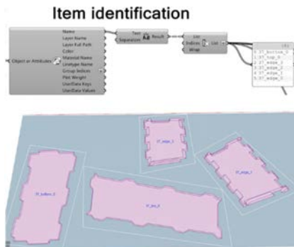
Figure 215. The second optimization stage mainly improves item tagging and referencing. nesting quality is however not better than in the first version thus the first version is kept.
