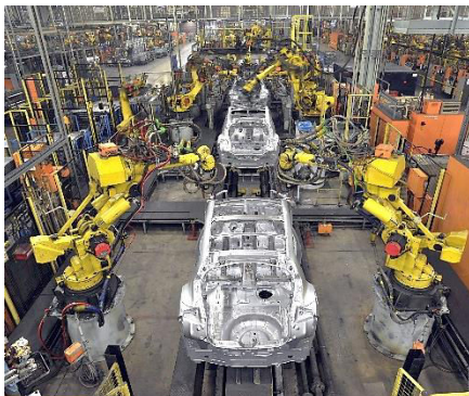
Figure 97. Industrial manipulators being used as welders in unattended mode at a Nissan Factory in Sunderland U.K. On: masonholden.wordpress.com/tag/carr-factory/
