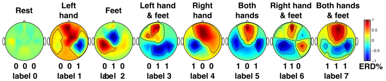
Fig. 5.4: Labeling convention. The proposed convention assigns a value of “1” to represent the sources that are active in terms of motor imagery-related activity; otherwise, the value corresponds to “0”. The number assigned independently to each source is used to generate a 3-bit word, whose decimal equivalence will be used when referring to each one of the classes considered in the paradigm. Note that the same convention is applied to the 4-class database, for which the sources associated to the left hand and right hand are used to generate a 2-bit word, where the less significant bit is associated to the use of the left hand, and the most significant bit to the use of the right hand.
