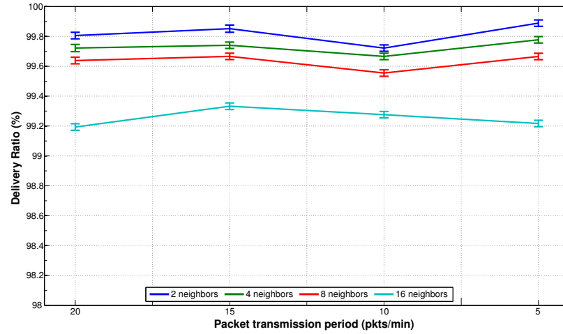
Figure 5.12: Global delivery ratio for different neighborhood sizes of node 2 (Fig.5.1(b)) with dynamic threshold.
