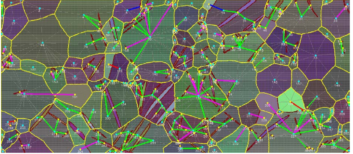
FIGURE 3.20 – Automatic output for a Zr EBSD map. The sample was cut from a high-purity clock-rolled Zr plate and loaded in compression along one of the in-plane directions up to 5% strain [11]. Yellow borders mark the grain joints, brown borders the twin joints. Green edges represent tensile 1 relation, magenta tensile 2, red compressive 1 and blue compressive 2.
