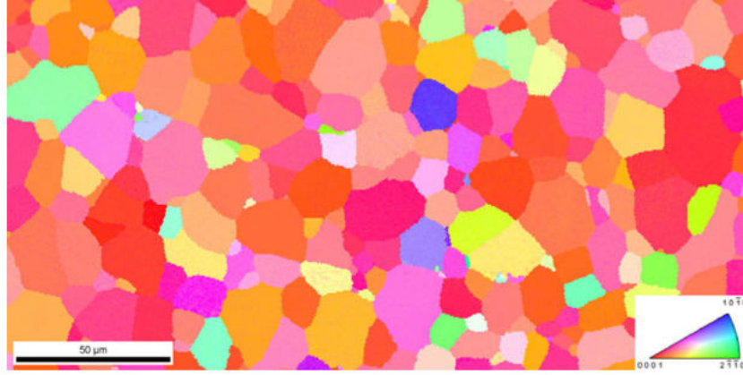
FIGURE 3.7 – Example of EBSD orientation map showing the undeformed microstructure of a high purity clock-rolled Zr specimen. Colors designate crystal orientations as indicated by the unit triangle in the bottom right-hand corner. The software used to generate this map is OIM Analysis [8].
