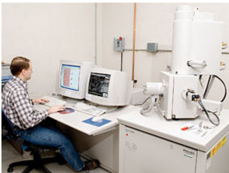
FIGURE 3.1 – Philips XL 30 F Orientation Imaging Microscopy System at Los Alamos National Laboratory, MST-6 (LANL web site).
