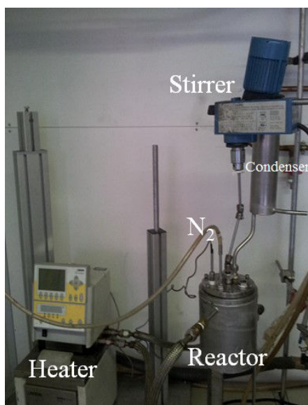
Figure 2.3 - Photo of reactor equipment of graft polymerization of styrene inside GTR particles
