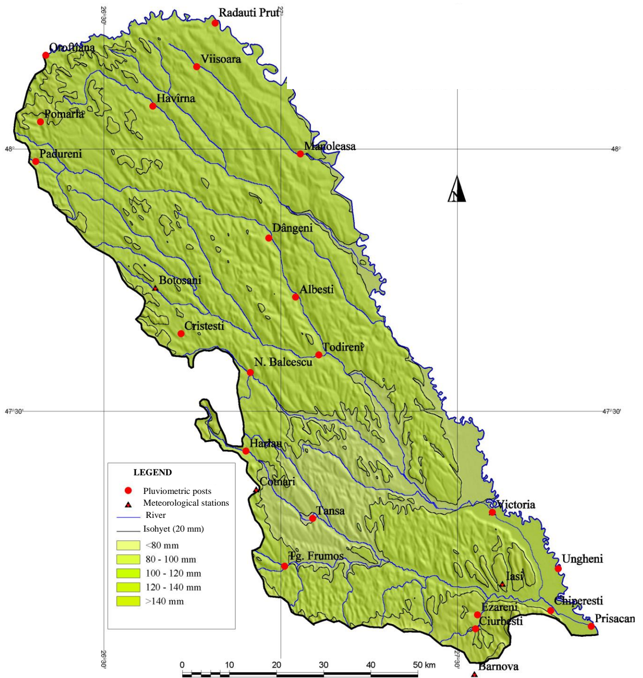
Fig. 5.17 Spatial distribution of multi-annual precipitation quantities in the autumn season in the 1991 – 2011 interval for the Moldavian Plain
