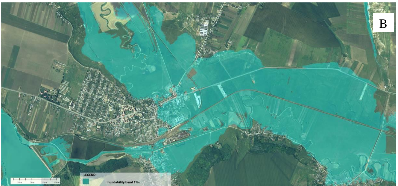
Fig. 6.60 Map extract – inundability band 1% (A); inundability band 1‰ (B) Bahlui river, Iloaia's Bridge
