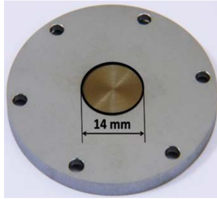
Figure 3.2: Tungsten sample and the molybdenum clamping ring used to mount the sample at Pilot and Magnum-PSI
